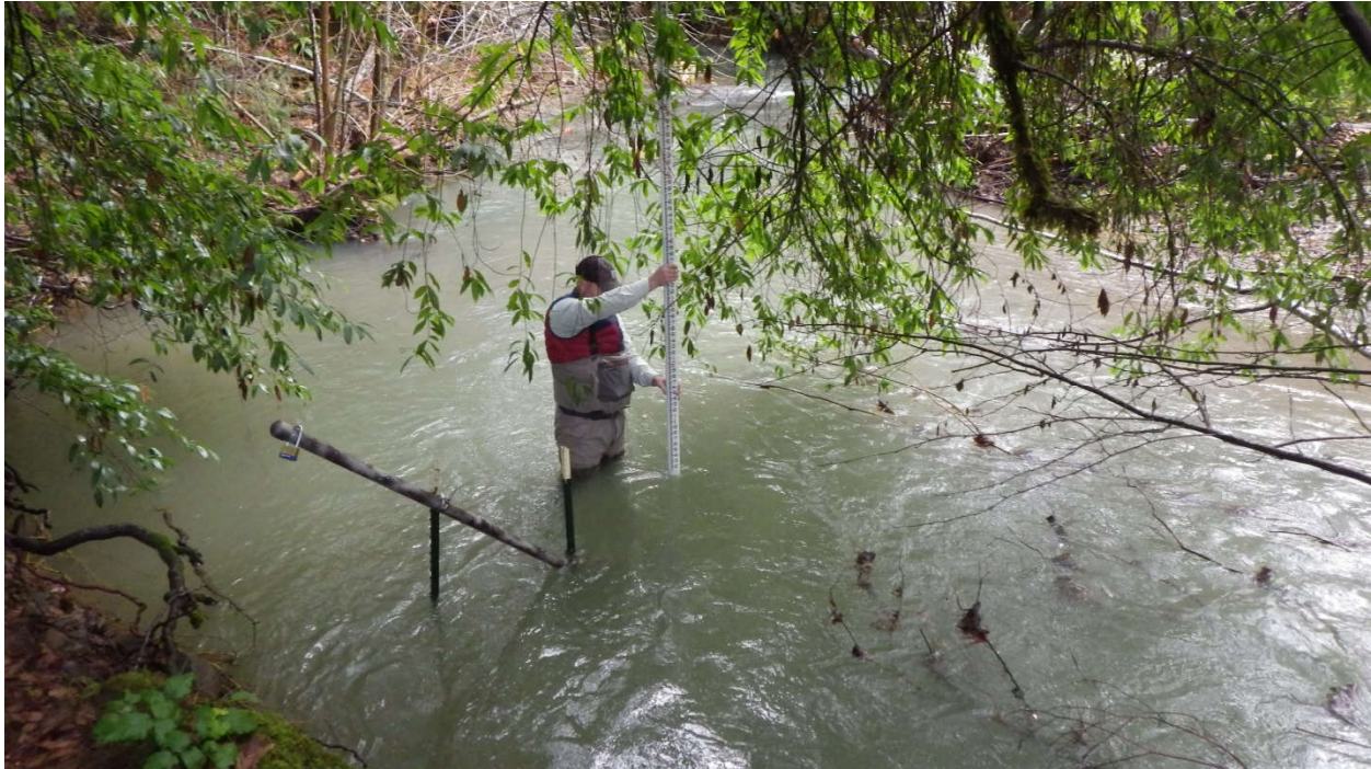
Figure 7. Water surface elevation survey above pressure transducer depth sensor.
