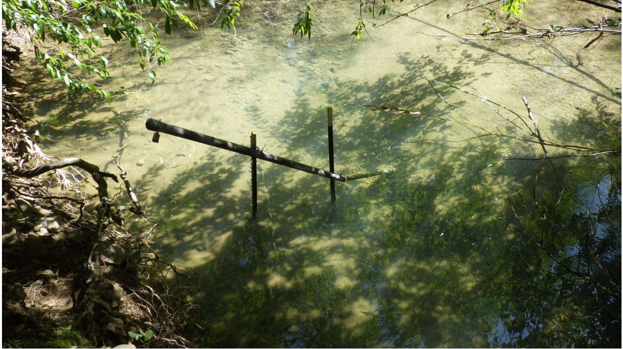
Figure 5. Typical pressure transducer stilling well installation.
