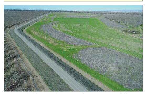
An innovative setback levee in Hamilton City reconnects the Sacramento River to its floodplain, creates habitat, and strengthens the failing J levee, originally built in 1906. The town has been evacuated six times in the last 25 years due to flood fears. The project is a collaboration of the US Army Corps of Engineers, local landowners, Reclamation District 2140, and The Nature Conservancy. Photo: The Nature Conservancy
