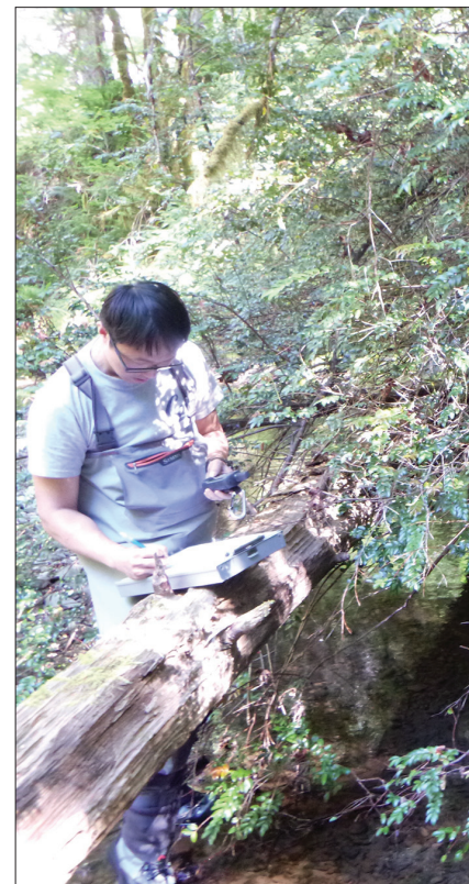
At McKee Creek, CDFW environmental scientist Jason Hwan installs a stilling well that contains a dissolved oxygen logger. The logger will be retrieved and readings will be downloaded at a later time.
