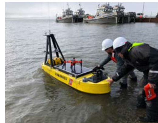
Fig 5. Unmanned vessel with UAS for oil spill sampling utilizing MPU5
