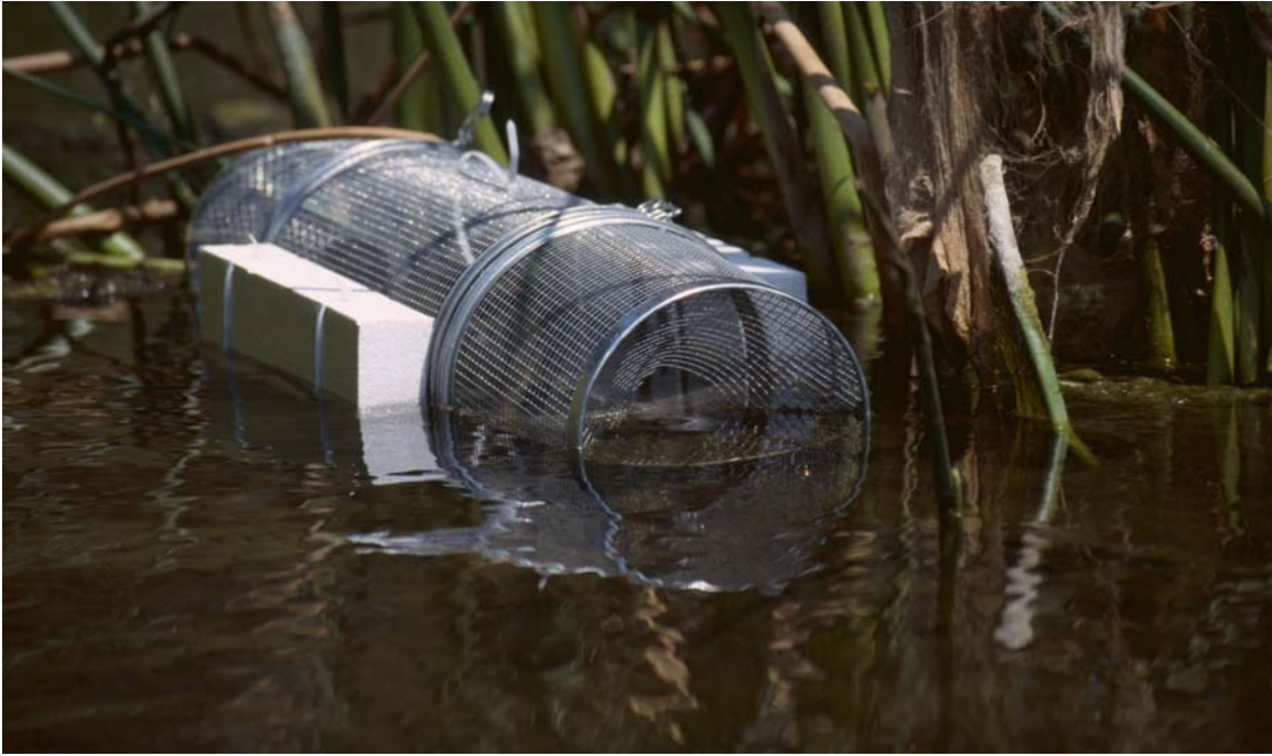
Figure 4. An aquatic funnel trap, designed originally to capture giant gartersnakes (Cassaza et al. 1999).
