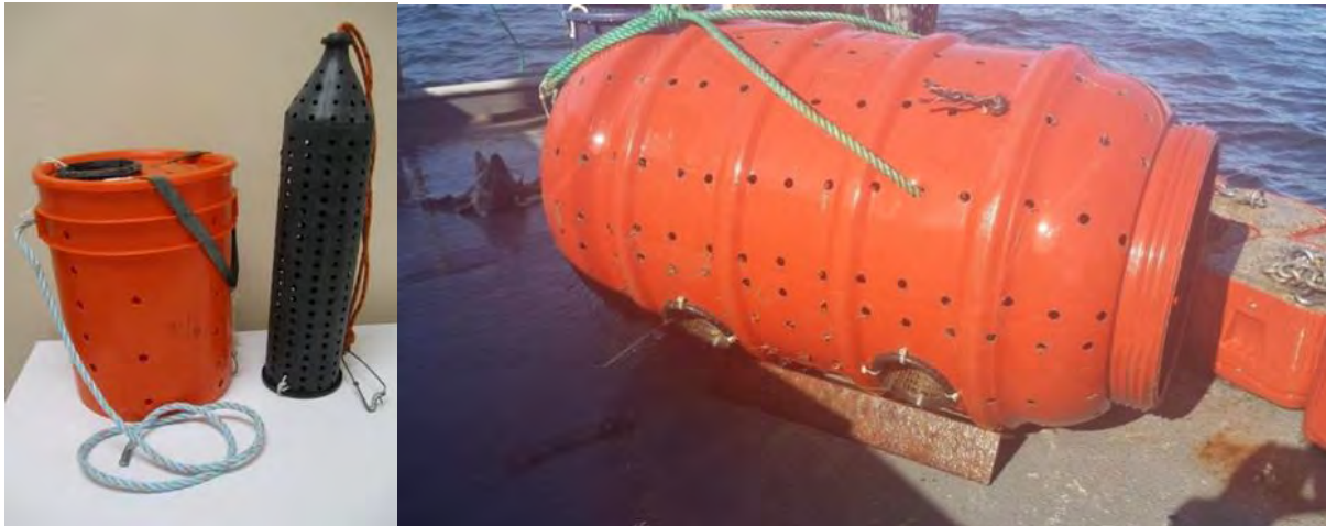
Figure 2-3. Five gallon bucket Hagfish trap, cylindrical Korean trap, and barrel trap (Photo Credit: Travis Tanaka, CDFW).
