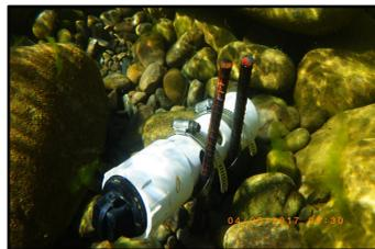
Pressure transducer in channel
