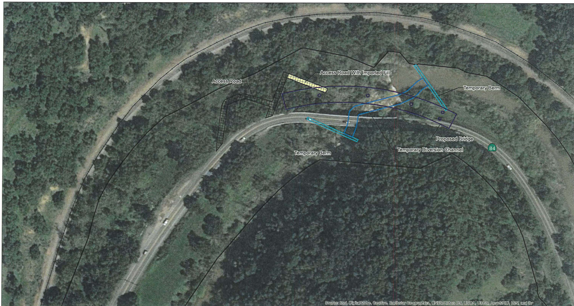
Figure 12: Access and Temporary Work Platform for Bridge Construction Alameda Creek Bridge Replacement Project EA 16030
