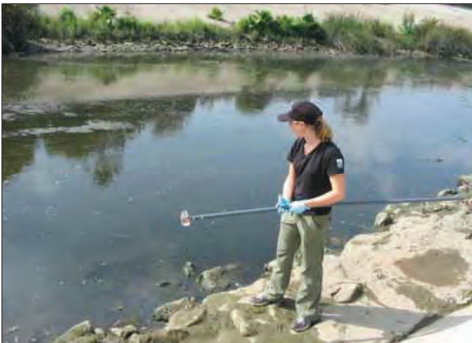
Lara Meeker extracts a sample of creek water for lab testing, taking measures to prevent contamination from anything on her hands, feet or clothing .
