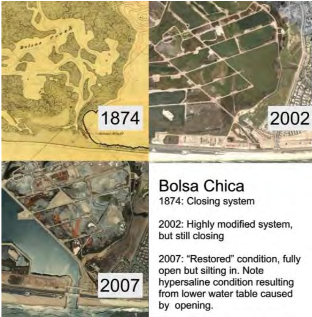
Figure 18. Creation of ahistoric conditions at Bolsa Chica through jettied a perennial deepwater channel. This "restoration" will require frequent and expensive dredging because existing physical processes do not support the fully open condition that was constructed. The areas surrounding constructed wetland appear to be drier and saltier because the water table will have dropped following complete opening.
