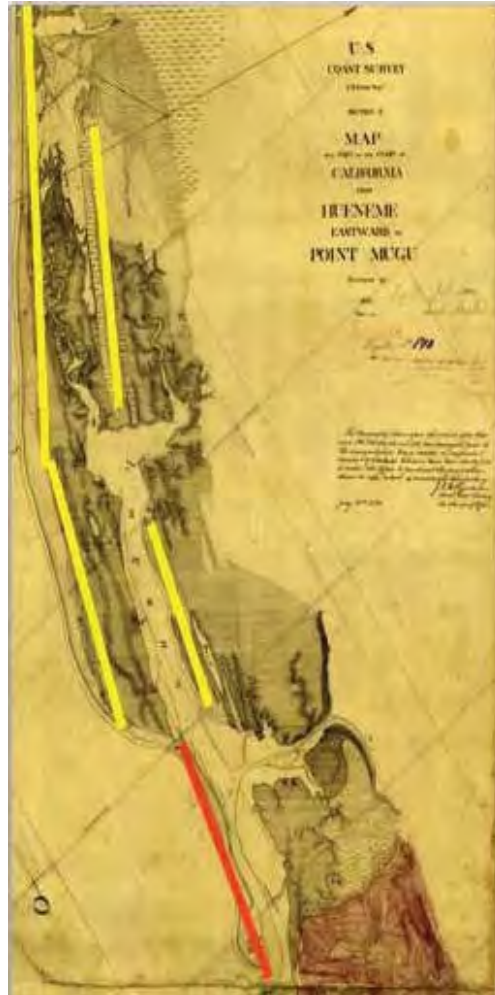
Figure 4. Series of barrier sand spits generating the prograding shoreline and forming much of the space of Mugu Lagoon (ca. 1860). Note the stable sand spits (yellow bars) apparently formed by a succession of longshore "trapping" events. Note also the thin spit (red bar) historically observed to undergo cycles of mouth migration, closure, and breaching as supported by observation, successive mapping, and air photography (see Warme 1971). In addition, the older Holocene inland spit is cross-cut by an outflow channel contributing to the estuary space. This cross cutting feature was apparently associated with flood distributary behavior of the Santa Clara River.
