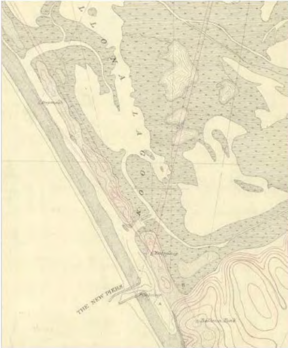
Figure 10. Detail of coastal survey (T-Sheet) from 1887 showing the new piers and entrance to proposed harbor.
