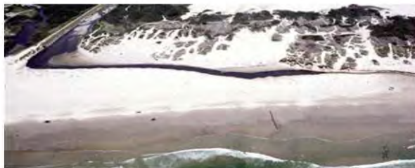
Arroyo Grande Creek, May 4, 1979. Closed high in the intertidal with a lagoon/channel feature paralleling the shore behind a beach ridge. This often occurs in high intertidal systems and in many systems late in the closure process.
