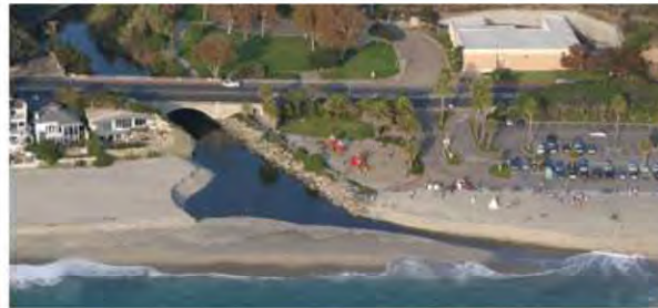
Aliso Creek (Orange County), Oct 23, 2004. Intertidal Closure. Note the steep North Side of the lagoon caused by a recent high stream flow event. The mouth is likely part way through the closure process.
