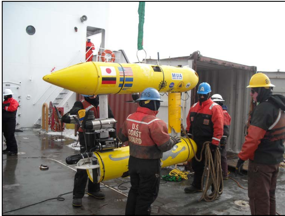
Figure 3. Jaguar AUV, representative of a lightweight AUV.
