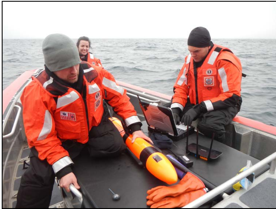
Figure 2. Riptide Micro-UUV, representative of man-portable AUV.
