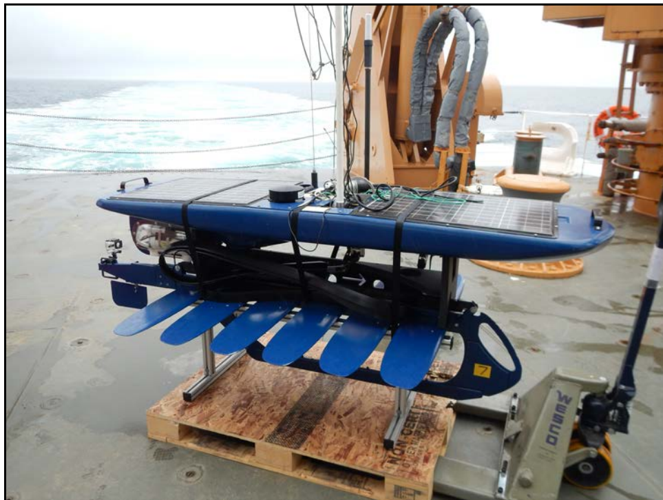
Figure 5. Wave Glider ready to be deployed off of USCGC HEALY during Arctic Shield 2014.
