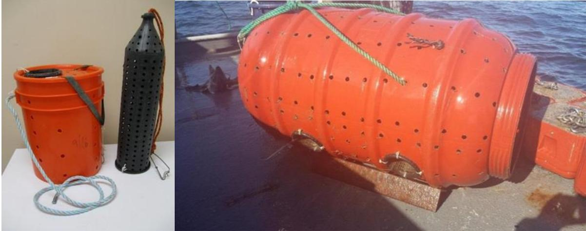
**Figure 2-2.** Five gallon bucket Hagfish trap, cylindrical Korean trap, and barrel trap (Photo Credit: Travis Tanaka, CDFW).
