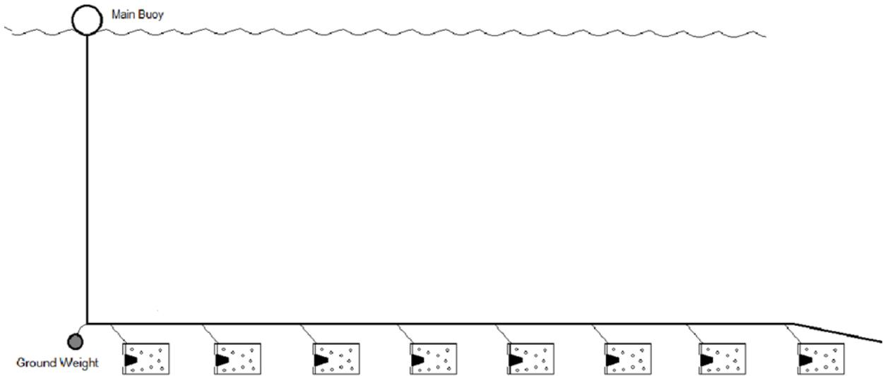
**Figure 2-3.** Graphic of a groundline equipped with Hagfish bucket traps (Illustration Credit: Ashok Sadrozinski, CDFW).
