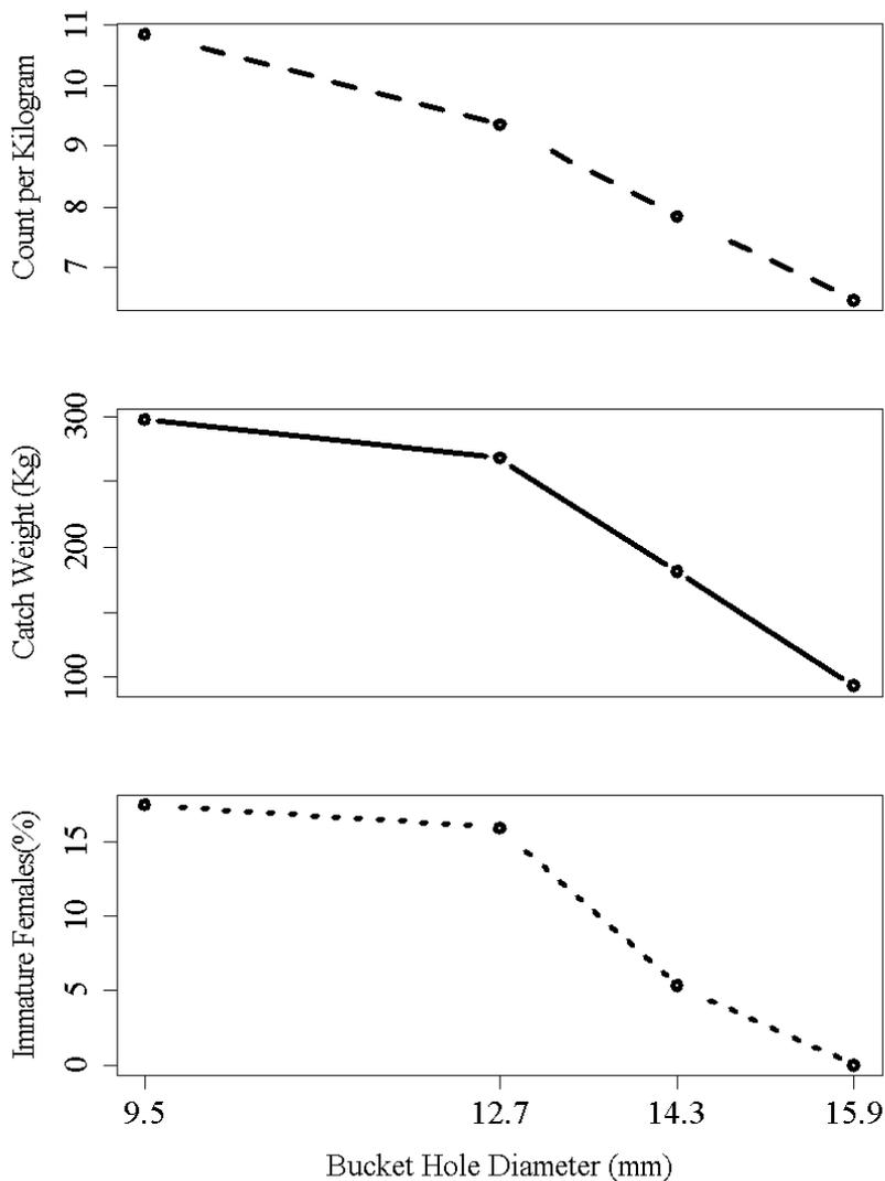
**Figure 4-3.** Results from a trap hole diameter study suggests holes 14.3 mm (0.56 in) in diameter are a compromise between retained catch and escape of immature female Hagfish (Reproduced from Tanaka and Crane 2014).
