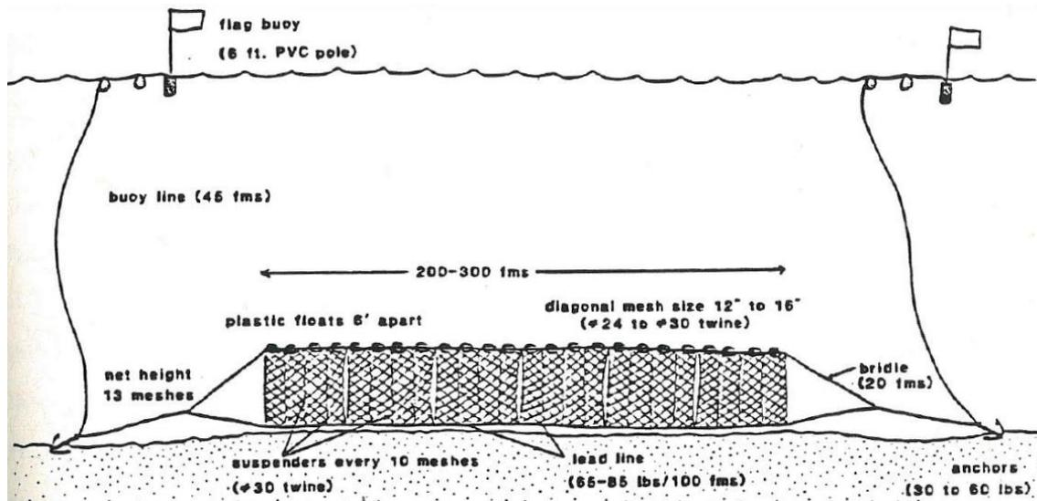
**Figure 2-2.** Illustration of a bottom set gill net anchored to the ocean floor as used in the Pacific Angel Shark fishery (Reproduced from Bedford 1987).
