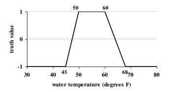
Figure 4. EMDS Reference Curve. EMDS uses this type of reference curve in conjunction with data specific to a stream reach. This example curve evaluates the proposition that the stream's water temperature is suitable for salmonids. Break points can be set for specific species, life stage, or season of the year. Curves are dependent upon the availability of data.
