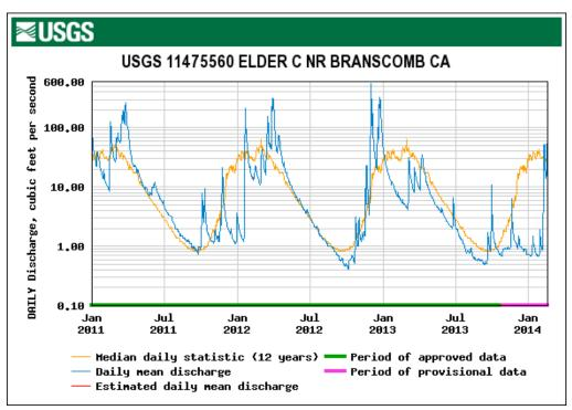
*Figure 49. Daily mean discharge (in cfs) and mean daily discharge (45-year average in cfs) for USGS gauging station at Elder Creek, showing 2011-2014 data.*
