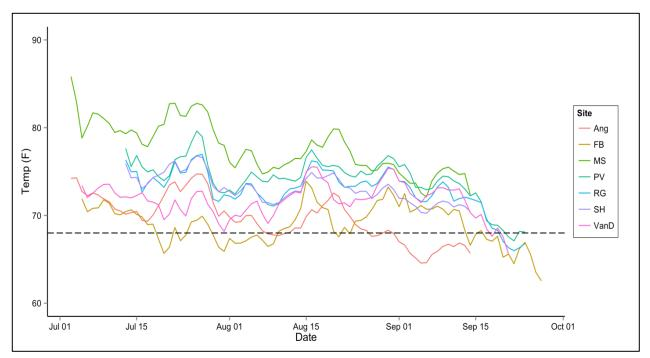
Figure 47. Daily average temperatures (degrees F) from July 3 through September 24, 2013, recorded at 7 sampling locations in the Eel River Basin. Data and graph provided by Keith Bouma-Gregson (UC Berkeley, 2014). Ang = Angelo Reserve; FB = Fernbridge; MS = Mainstem Outlet Creek; PV = Phillipsville; RG = Richardson Grove; SH = Standish-Hickey SRA; VanD = Van Duzen River.
