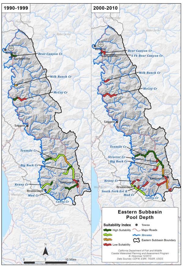
Figure 41. Pool depth suitability in SF Eel River Eastern Subbasin streams, using data collected between 1990 and 1999, and 2000 and 2010.
