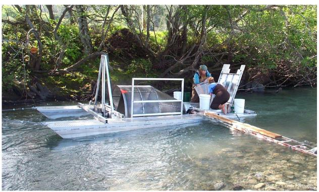
Figure 38. Rotary screw trap used to sample outmigrant juvenile fish.
