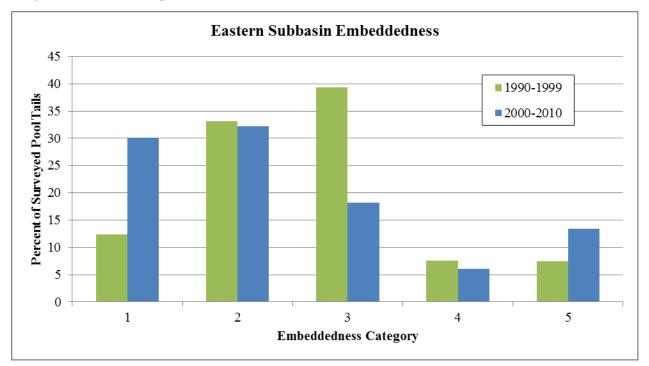
Figure 43. Cobble Embeddedness in the Eastern Subbasin, using data collected from 1990-1999 and 2000-2010.
