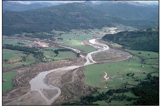
Figure 10. Confluence of Yager Creek with Van Duzen River. Note channel widening and bank erosion in the Van Duzen River linked to sediment inputs and high flows from Yager Creek. Photo courtesy of Kris Coho.
