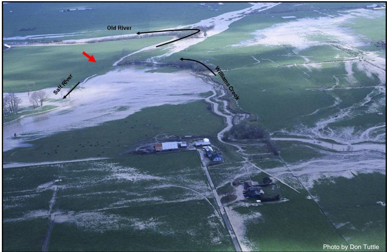
Figure 11. Williams Creek, Salt River and the Old River in February 2004. Red arrow indicates the sediment plug in the Salt River at river mile 7.5.
