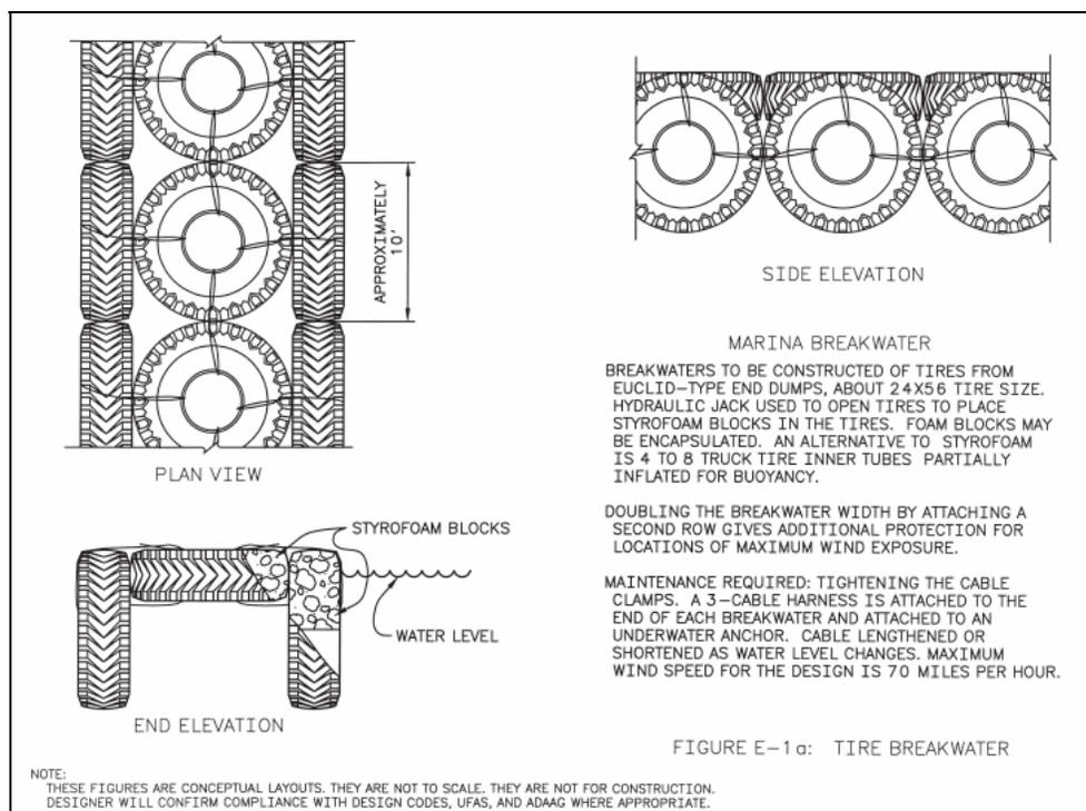
**Fig. 36. Tire structure breakwater design from the Bureau of Reclamation**
