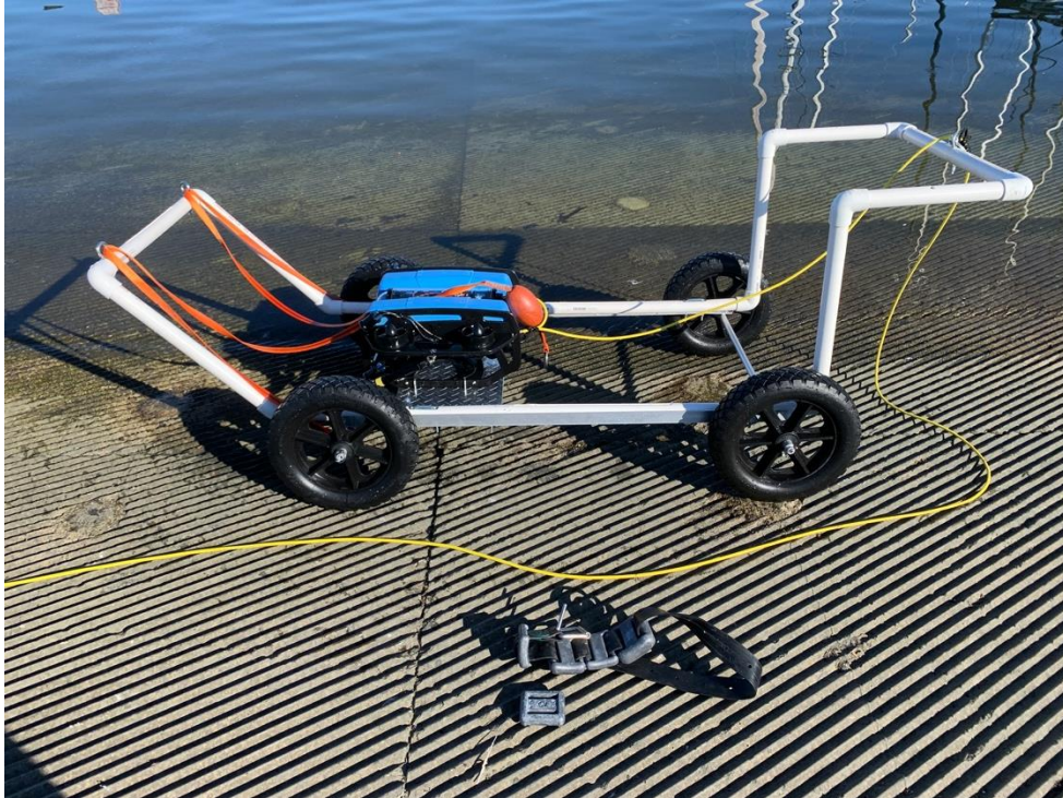
ROV Mounted to Tow Vehicle for Performing Bottom Survey at the SB Harbor Launch Ramp
