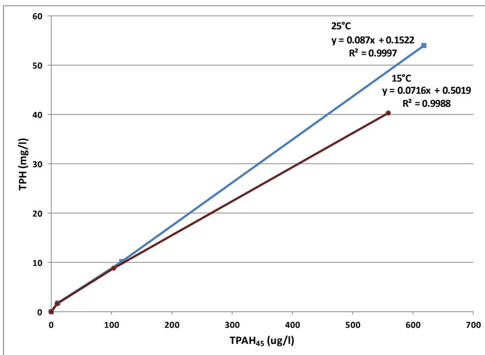
Figure 1. Relationship between total petroleum hydrocarbons (TPH mg/l) and total PAHs (TPAH<sub>45</sub> µg/l) for water accommodated fraction dilutions prepared at 25°C and 15°C.
