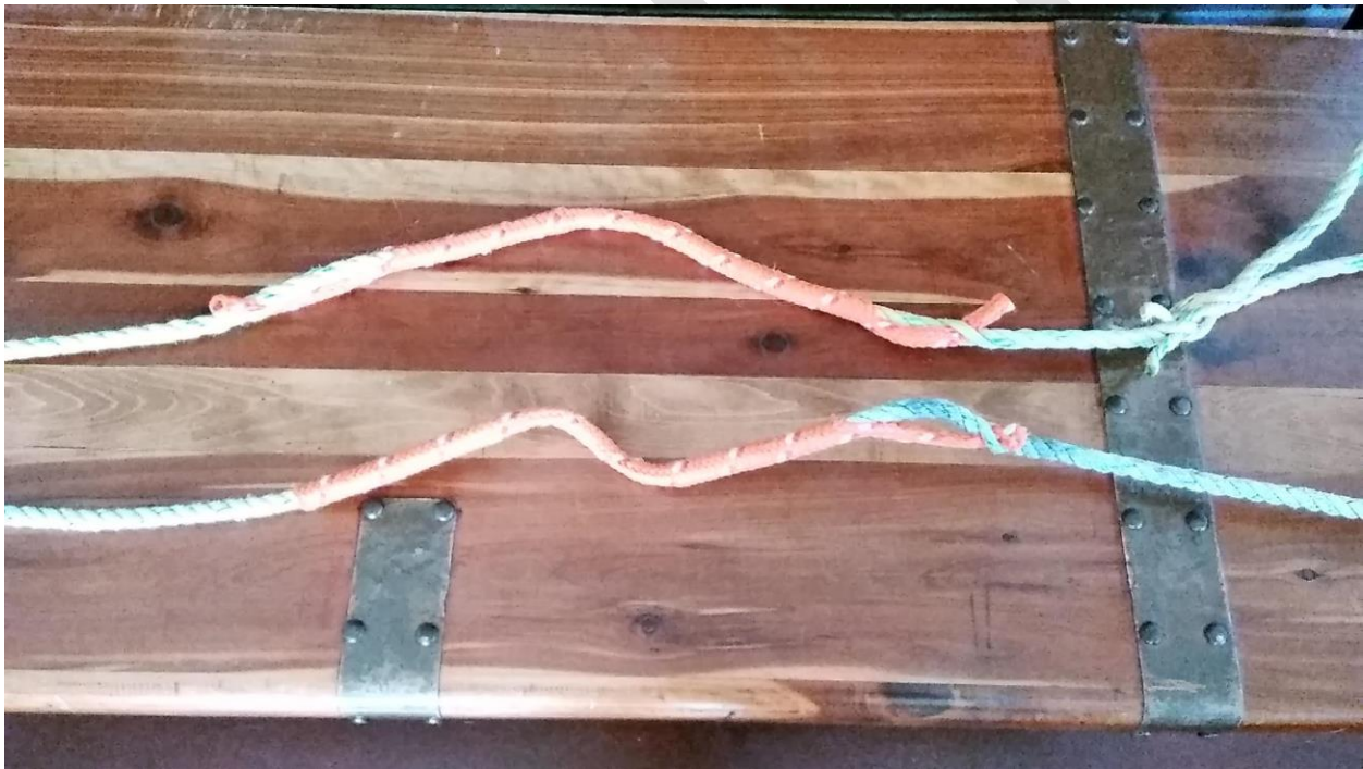
Figure 5-2. Novabraid Yale grip sleeve, courtesy of Fran Recht (Pacific States Marine Fisheries Commission).
