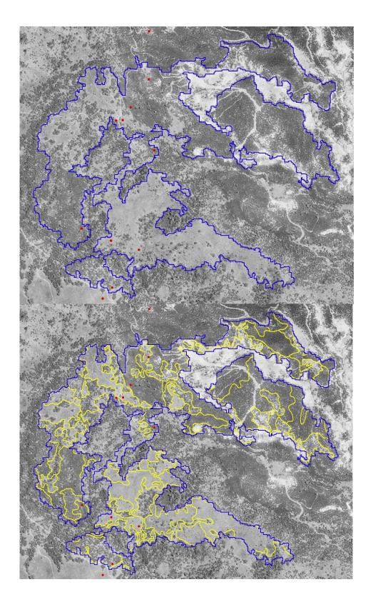
**Figure 8.** Example of medium-scale map with one large polygon mapped as Lower Elevation Mixed Chaparral habitat (blue polygon in first picture) within which the fine-scale map had 323 polygons with 21 different alliances and habitats mapped (yellow polygons in second picture). Scale was 1:6,600.
