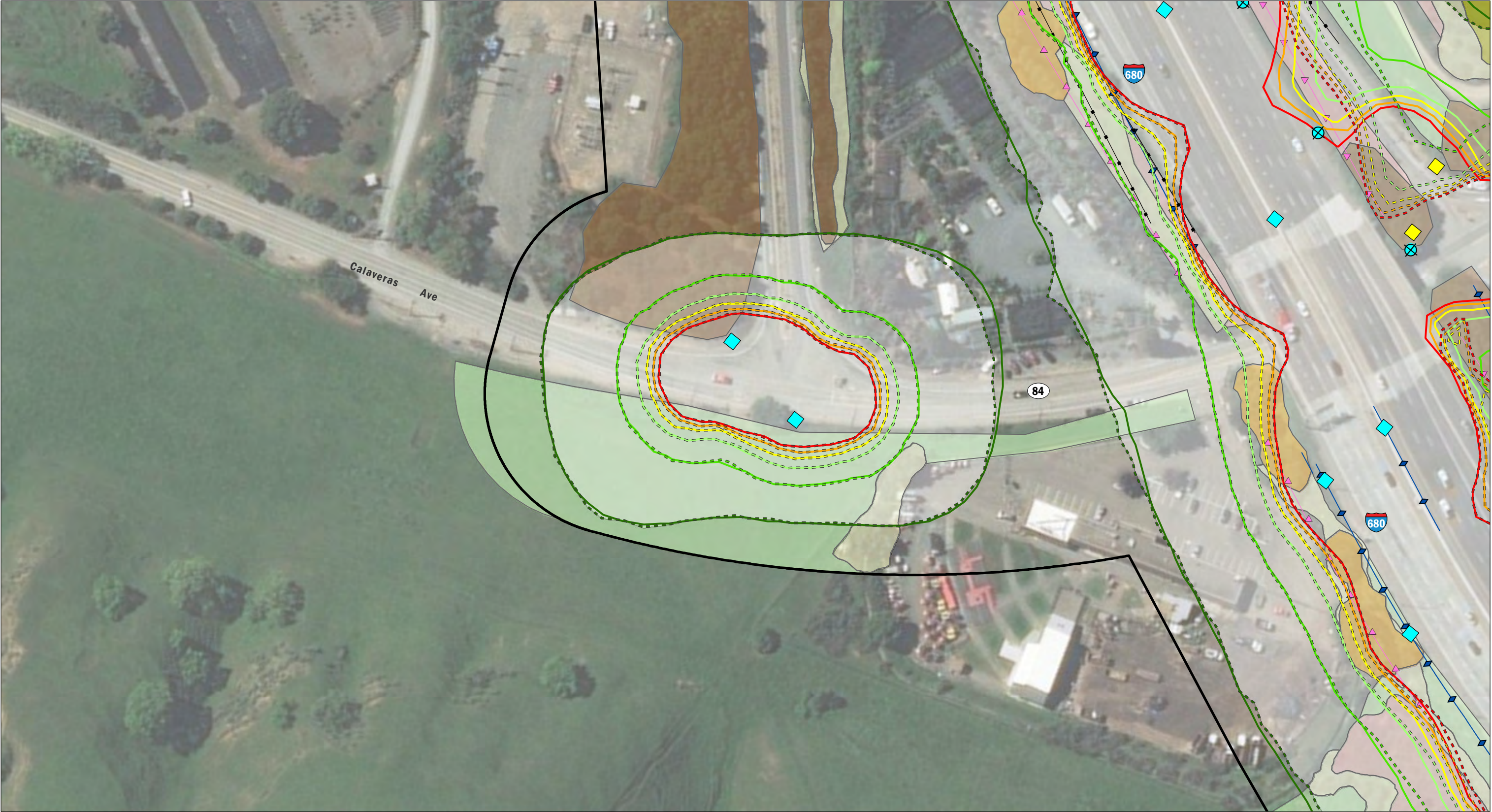
FIGURE 1A Proposed Low Lux Lighting Isolines - No Backside Shielding Page 5 of 15
