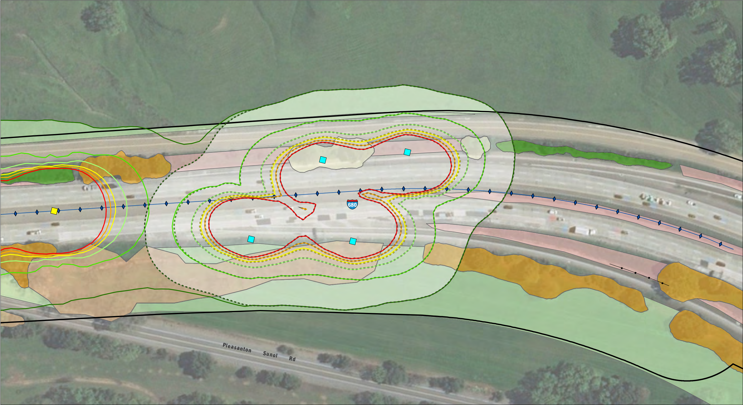
FIGURE 1A Proposed Low Lux Lighting Isolines - No Backside Shielding Page 12 of 15
