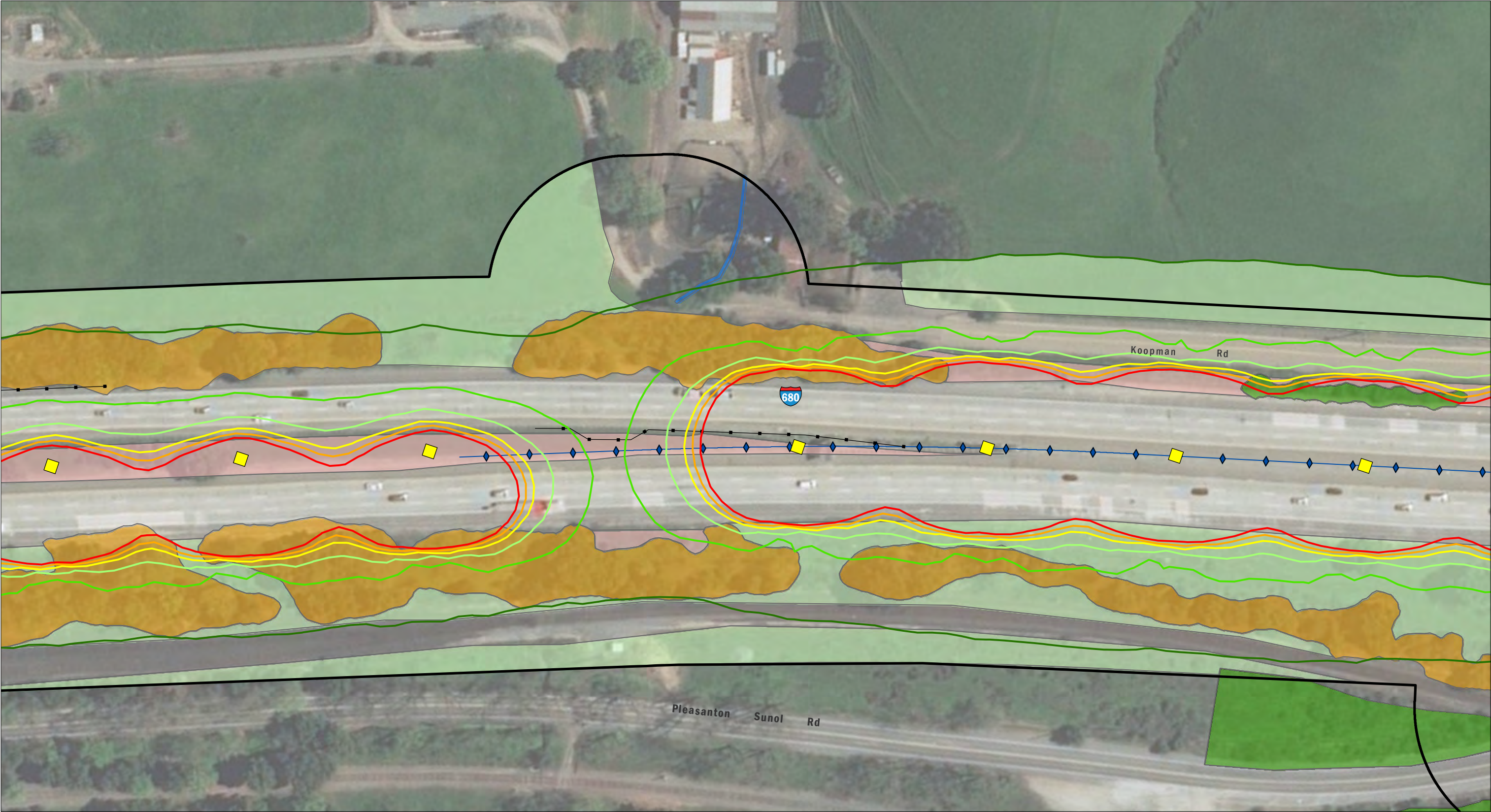
FIGURE 1A Proposed Low Lux Lighting Isolines - No Backside Shielding Page 14 of 15
