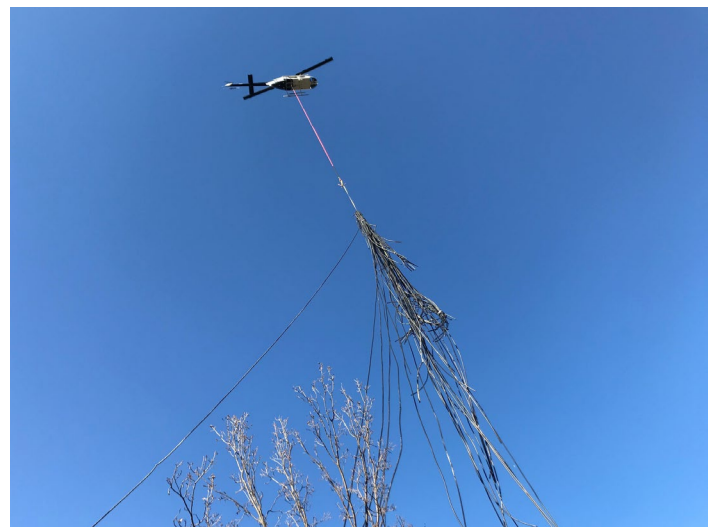
Airlift cleanup of polypiping from an illegal grow at the Tehama Wildlife Area. Remote areas are especially difficult to clean up and such efforts cost thousands of dollars.
