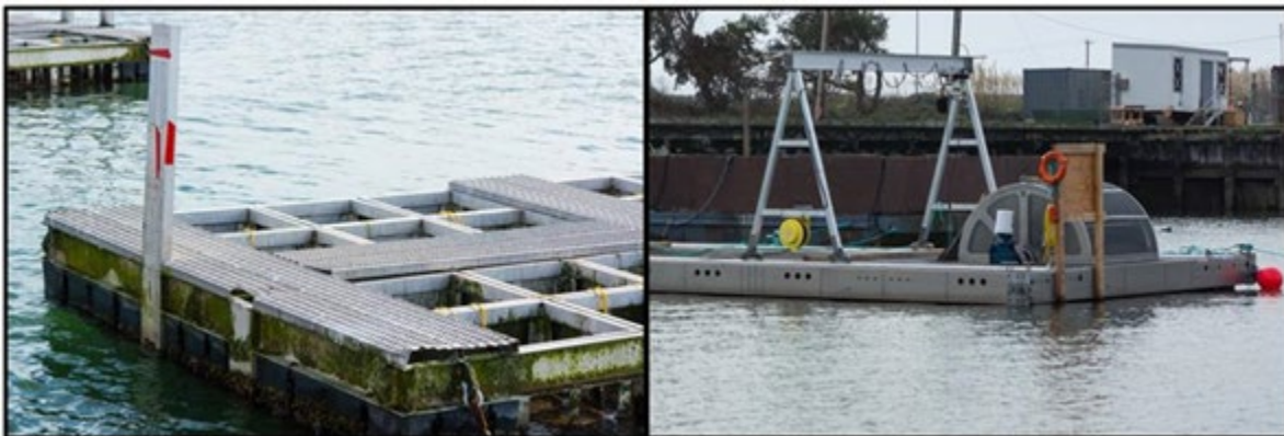
Figure 2-12. Raft modification: floating upwelling raft system. Upwelling containers hang in compartments on floating rafts (left) with a large paddle wheel directing nutrient rich water through containers (right) (Photos: CDFW).
