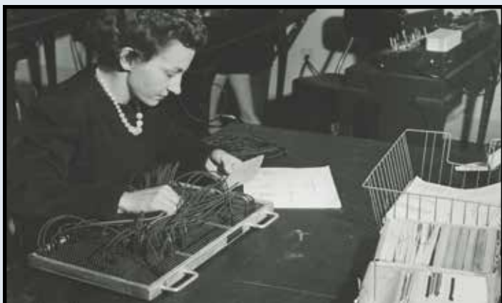
1937 control panel for tabulating.
