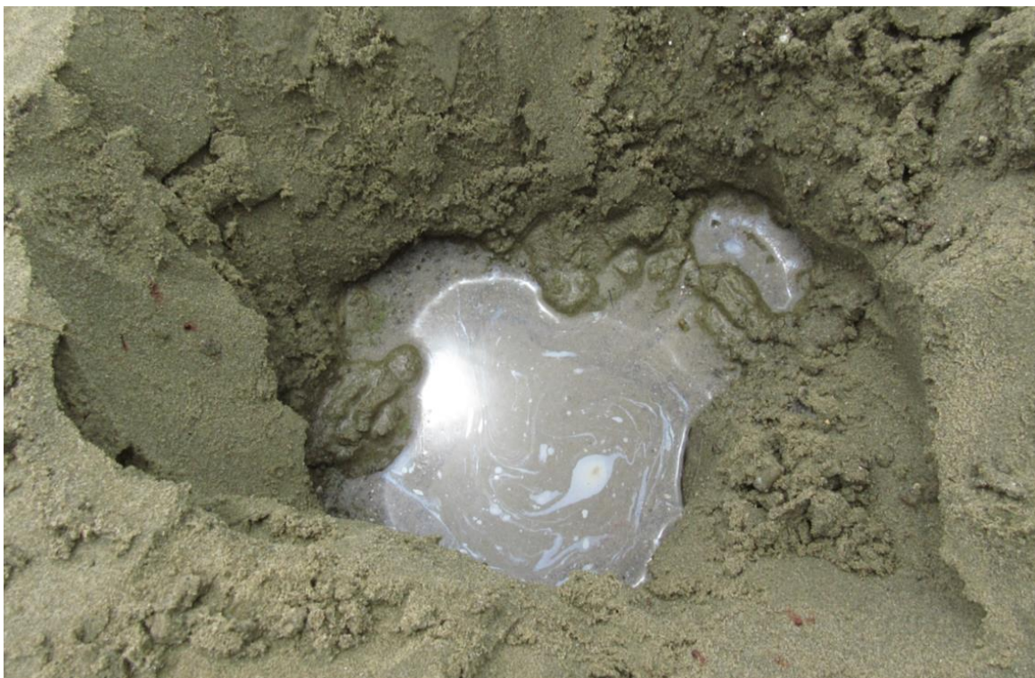
Figure 9. Sediment porewater sample location showing oil sheen on the surface. Photo Credit: Natural Resource Damage Assessment Trustees.
