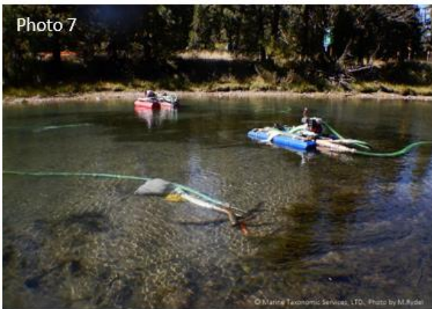
Photo 6. Diver-assisted suction removal of Eurasian watermilfoil (diver not shown).
