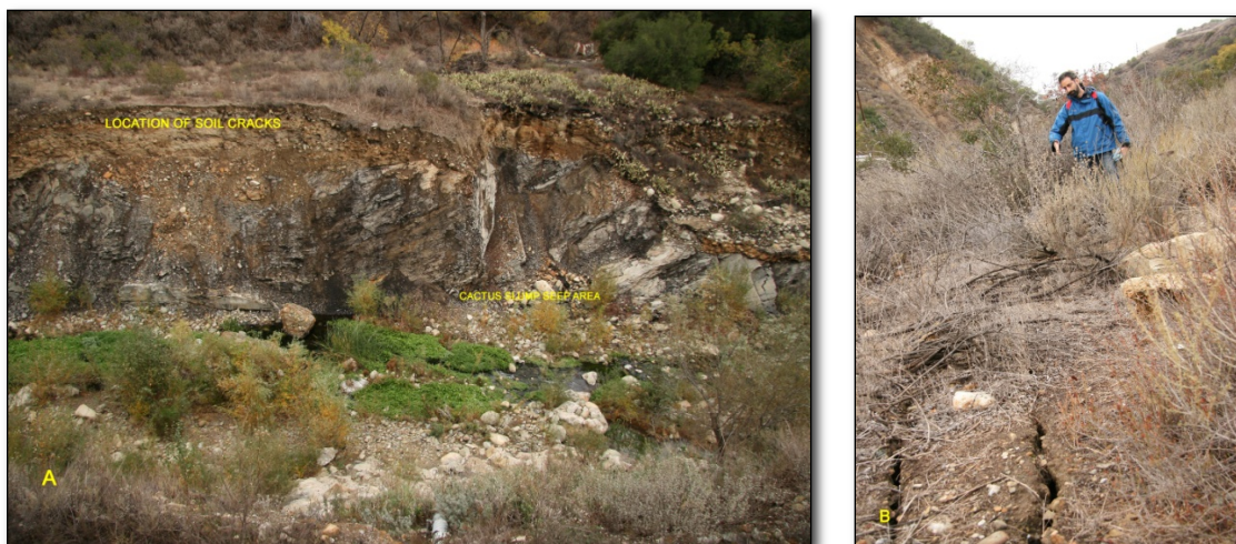
Fig. 35. Left) Location of unstable soil and cracks. Right) Examples of soil fissures at top of bank just upstream of the Cactus Slump Seep Area.
