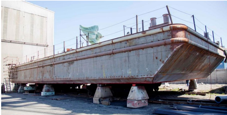
Figure I-4. Flat Top Construction Barge with Characteristic Tapered Ends
