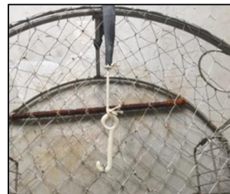
Round-style crab trap with plastic hook attached by the destruct device. The lid will open when the device corrodes or fails. Photo by J. Langell and J. Hendricks, CDFW
