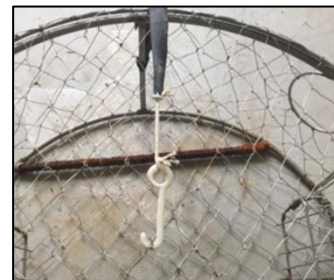
Round-style crab trap with plastic hook attached by the destruct device. The lid will open when the device corrodes or fails. Photo by J. Langell and J. Hendricks, CDFW
