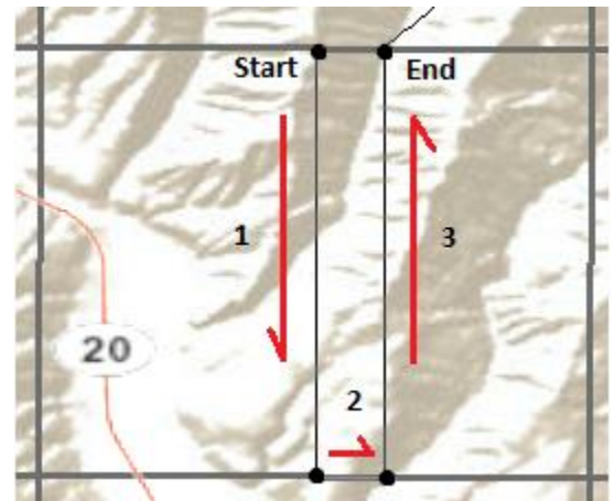
Figure A3 Close up of a mirrored linear transect skeleton within a 2km x 2km grid cell; numbers indicate order of transect, arrows indicate direction of travel; each black point indicates the start/end point of a segment with the transect start/end points labeled as such
