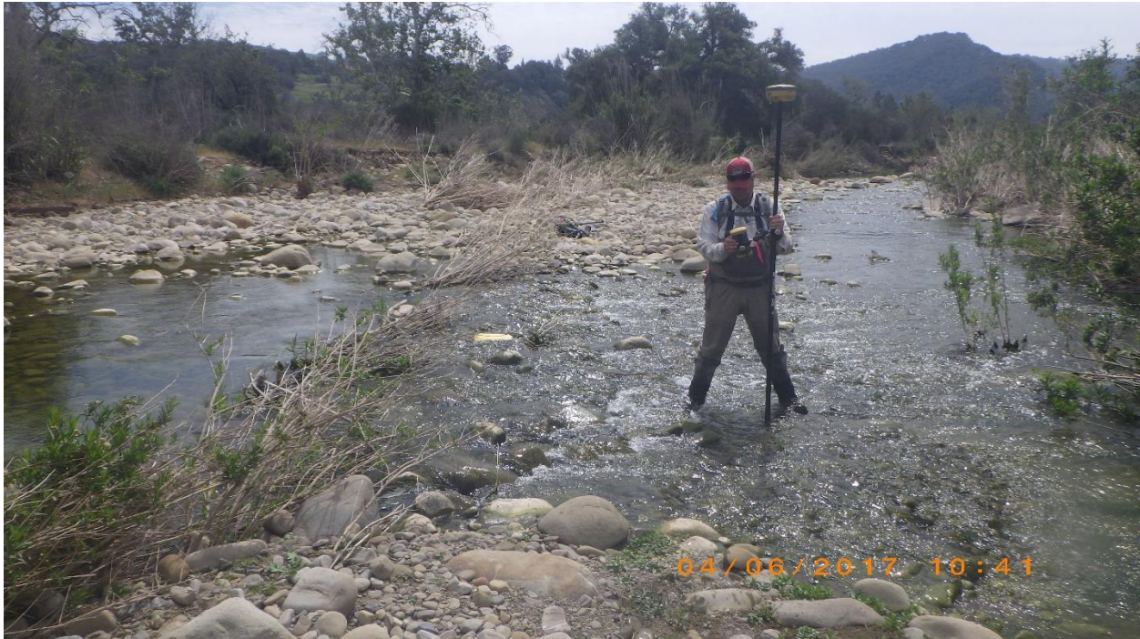
Figure 18. Surveying points across a riffle in the Ventura River intermittent reach study site. Riffle R15, downstream view at approximately 17 cfs.
