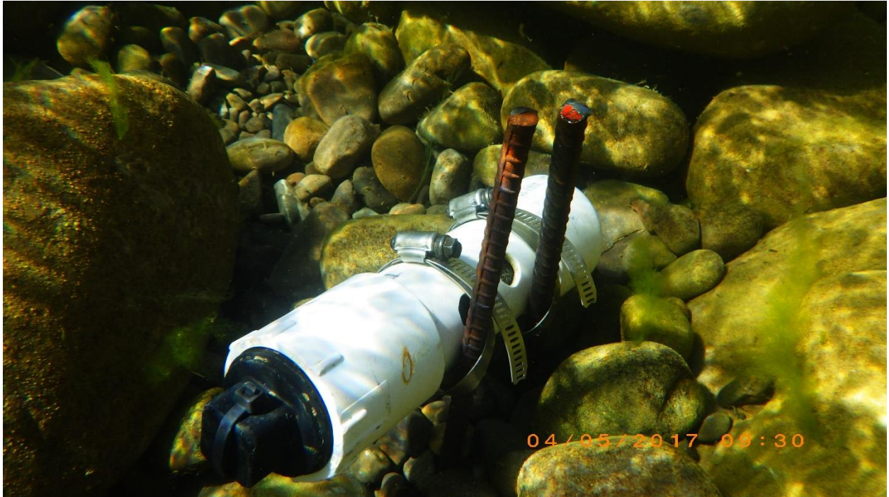
Figure 16. Post-storm PT6b installation near the upstream boundary.
