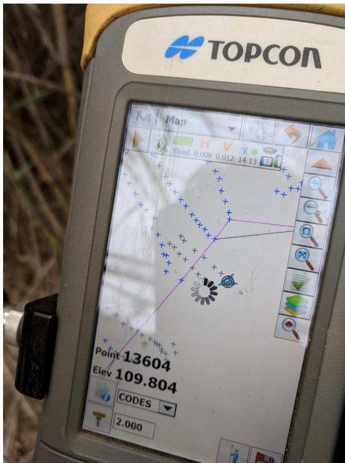
Figure 14. RTK GPS rover handheld data collector showing bed topography data points.
