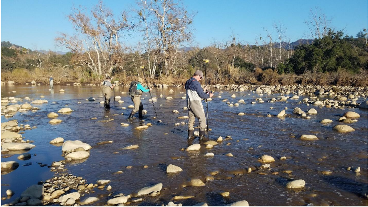
Figure 12. Collecting terrain model data in the study site using RTK GPS.
