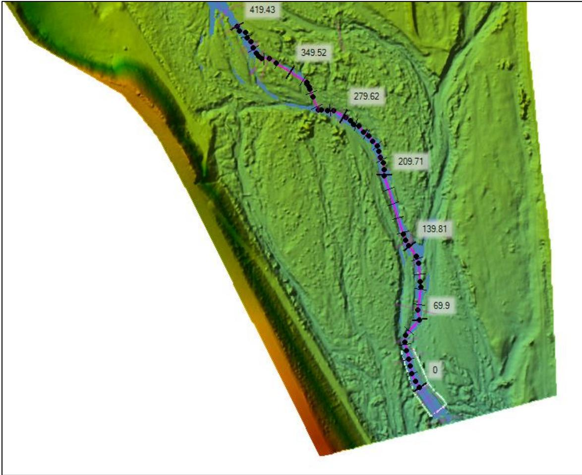
**Figure C-14.** Post-storm model depth validation locations overlain on 2018 QL1 LIDAR DTM at a simulated flow level of 17 cfs (distances in meters).
