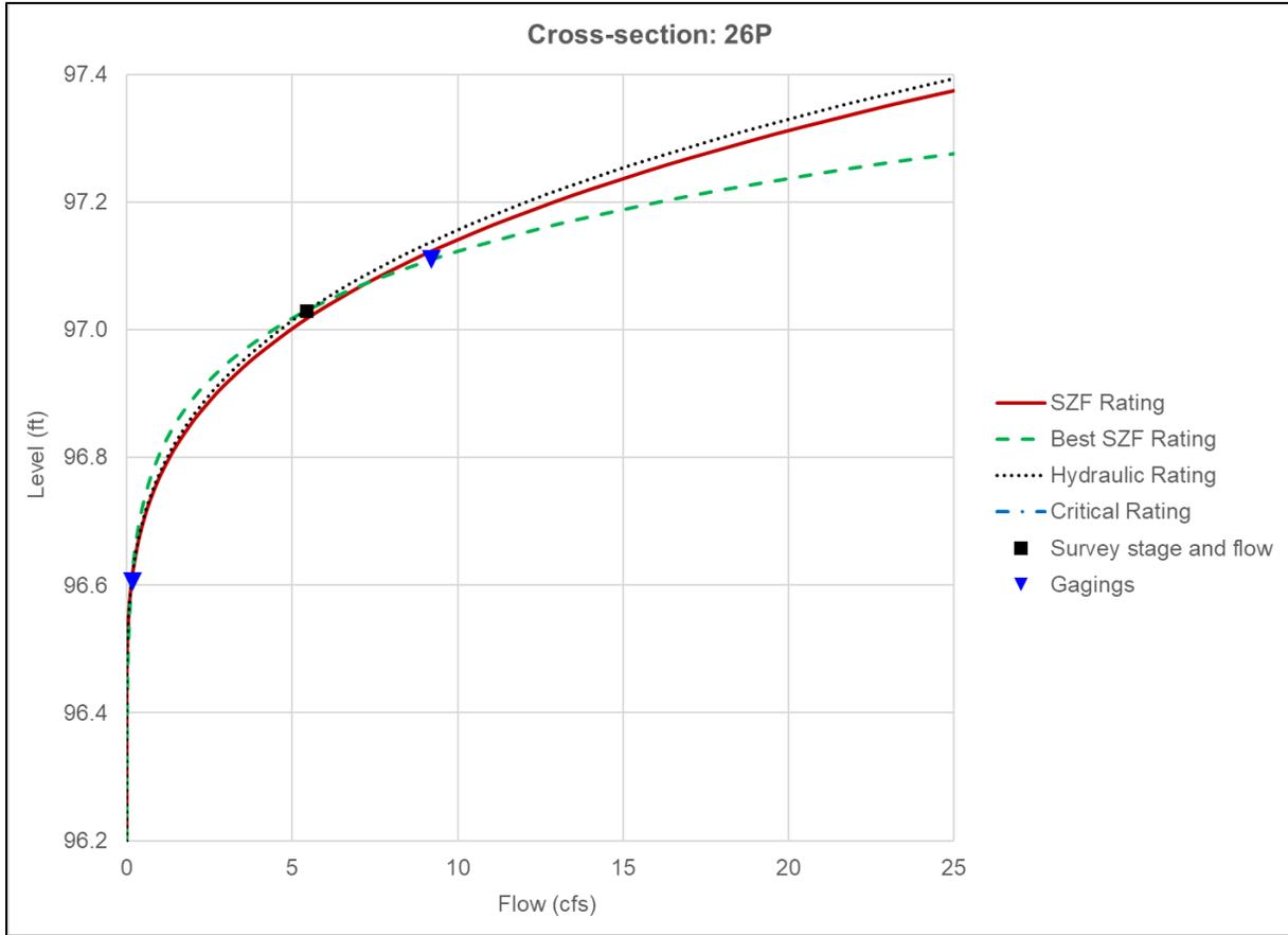
**Figure B-3.** Rating curve outputs for Reach 1, cross section 26P. This rating curve also appears as an example in Appendix A.
