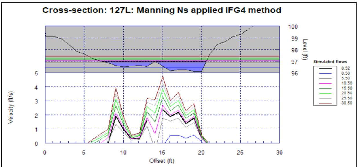
**Figure D-21.** Cross section 127L after VDF modification at simulated flows ranging from 0.5 cfs to 30.5 cfs.
