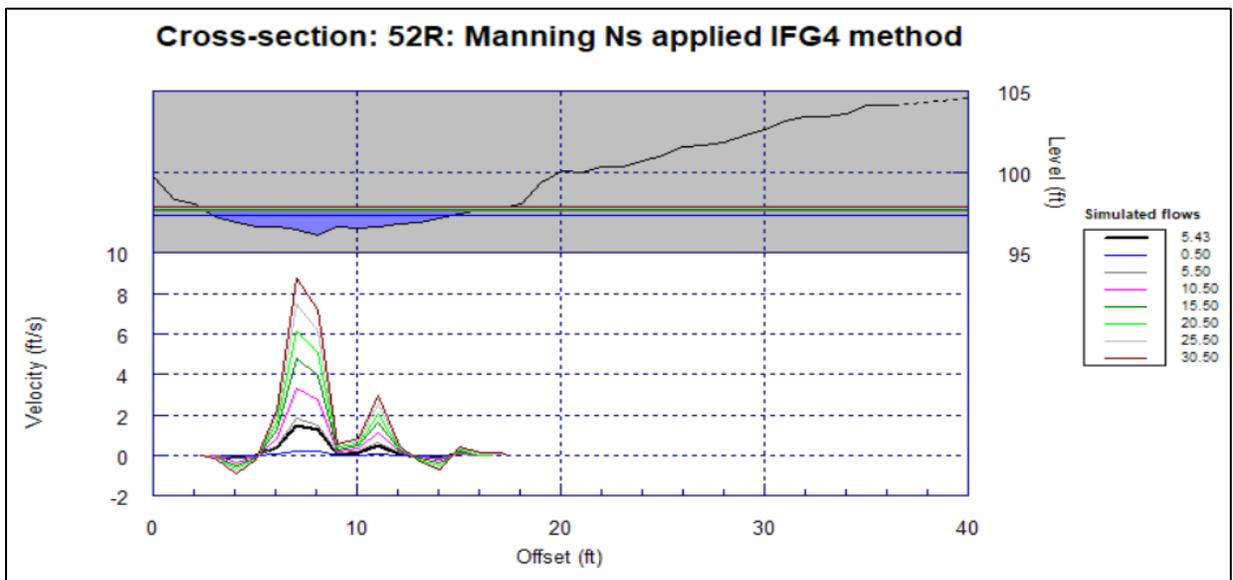
**Figure D-9.** Cross section 52R at simulated flows ranging from 0.5 cfs to 30.5 cfs.
