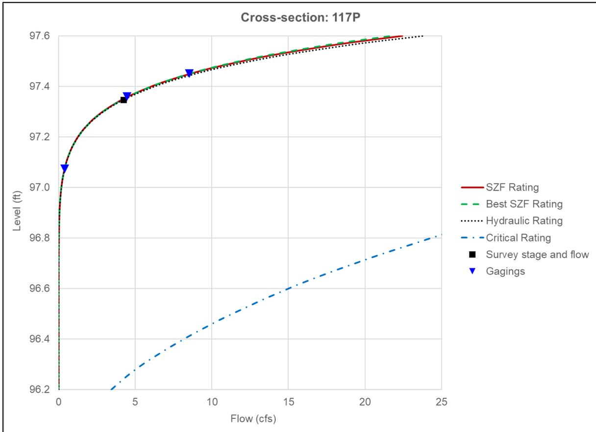
**Figure B-14.** Rating curve outputs for Reach 2, cross section 117P.
