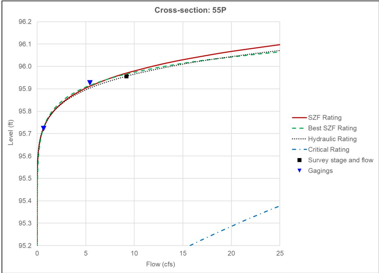
**Figure B-9.** Rating curve outputs for Reach 1, cross section 55P.
