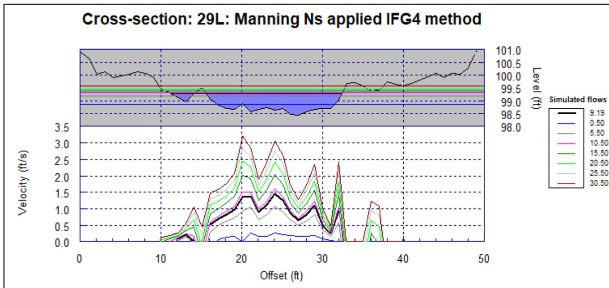
**Figure D-4.** Cross section 29L at simulated flows ranging from 0.5 cfs to 30.5 cfs.
