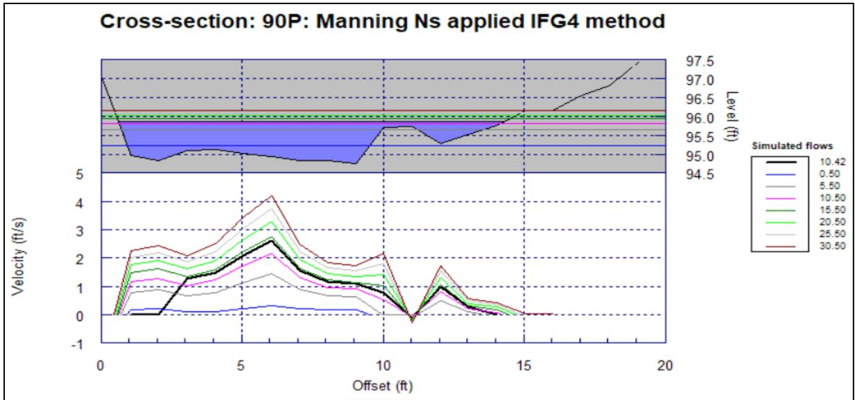
**Figure D-14.** Cross section 90P before VDF modification at simulated flows ranging from 0.5 cfs to 30.5 cfs.
