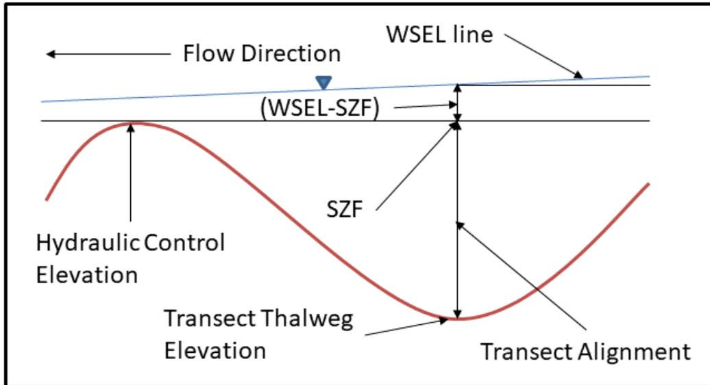
**Figure A-3.** Stage of zero flow (SZF) diagram.
