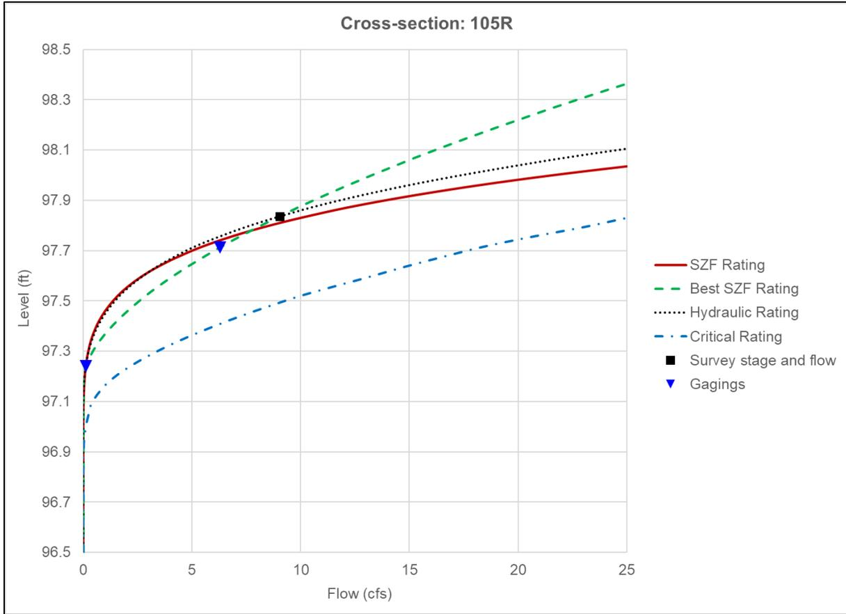
**Figure B-13.** Rating curve outputs for Reach 2, cross section 105R.
