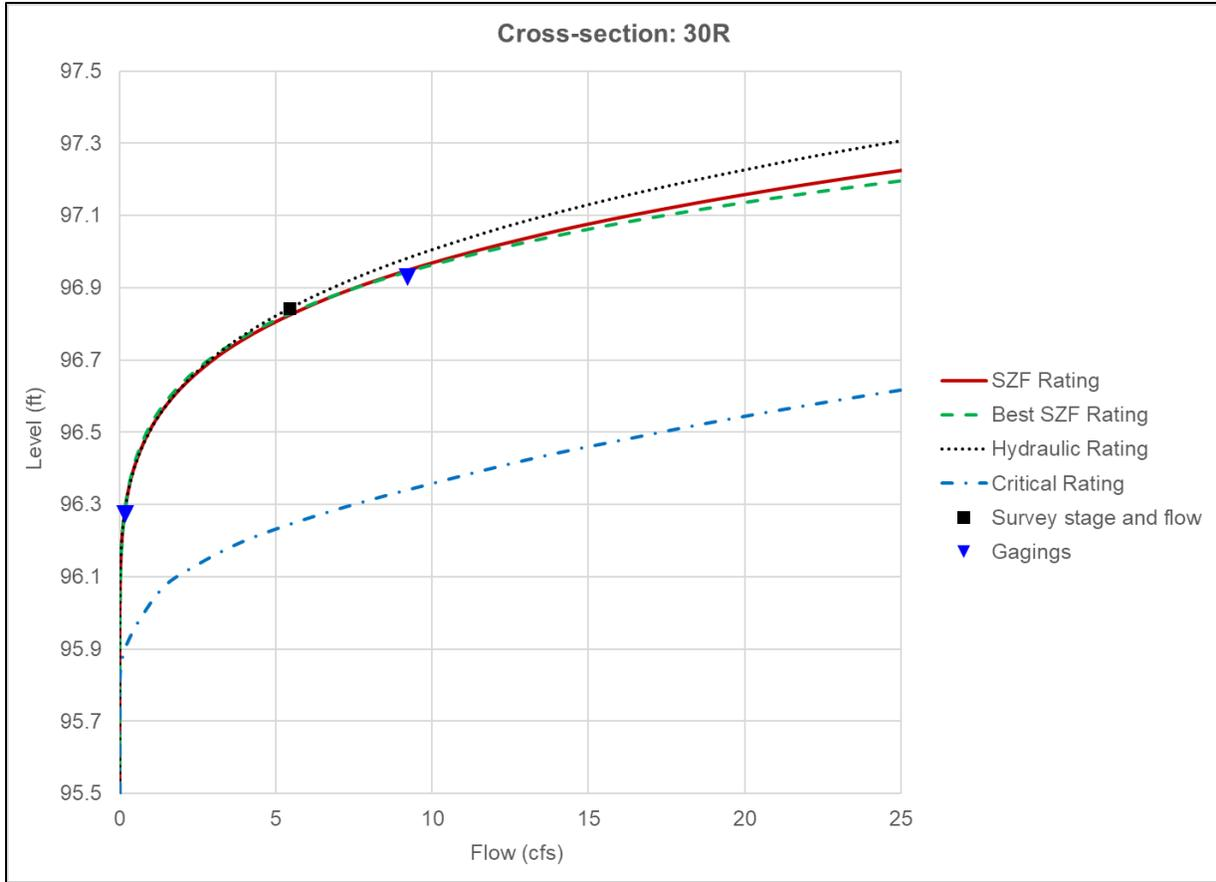
**Figure B-5.** Rating curve outputs for Reach 1, cross section 30R.
