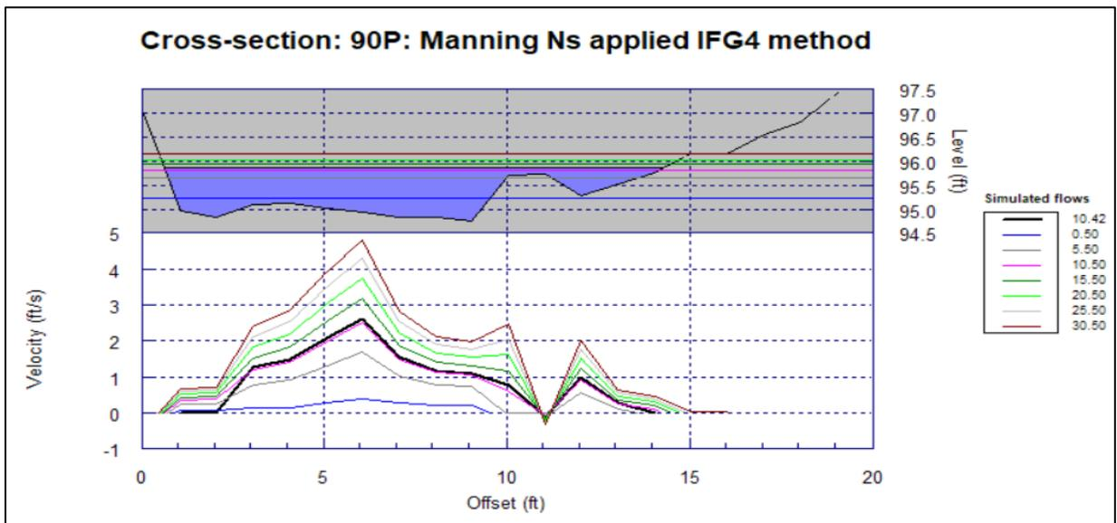
**Figure D-15.** Cross section 90P after VDF modification at simulated flows ranging from 0.5 cfs to 30.5 cfs.
