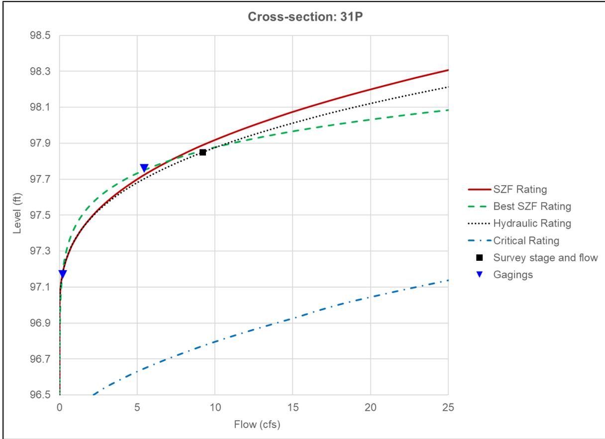
**Figure B-6.** Rating curve outputs for Reach 1, cross section 31P.
