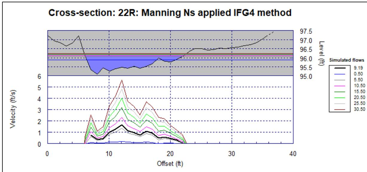
**Figure D-1.** Cross section 22R at simulated flows ranging from 0.5 cfs to 30.5 cfs.
