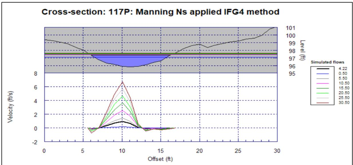
**Figure D-19.** Cross section 117P after VDF modification at simulated flows ranging from 0.5 cfs to 30.5 cfs.
