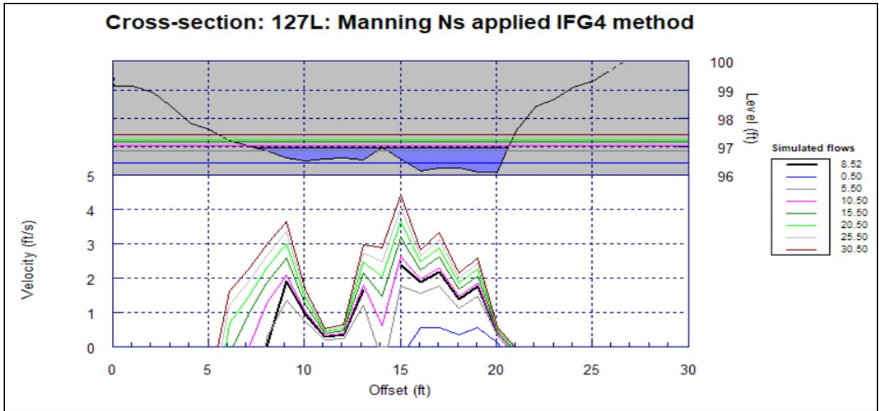
**Figure D-20.** Cross section 127L before VDF modification at simulated flows ranging from 0.5 cfs to 30.5 cfs.
