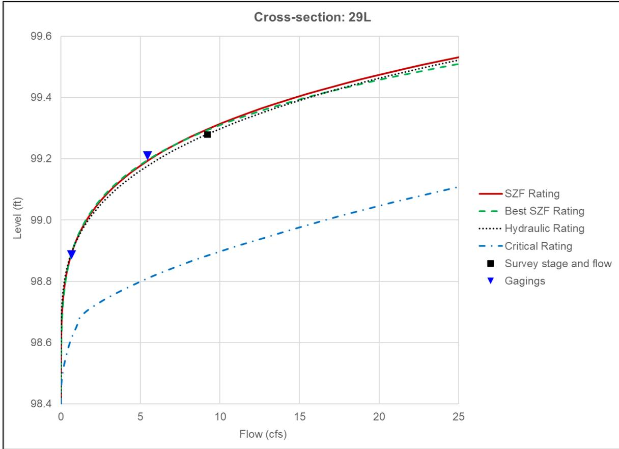
**Figure B-4.** Rating curve outputs for Reach 1, cross section 29L.
