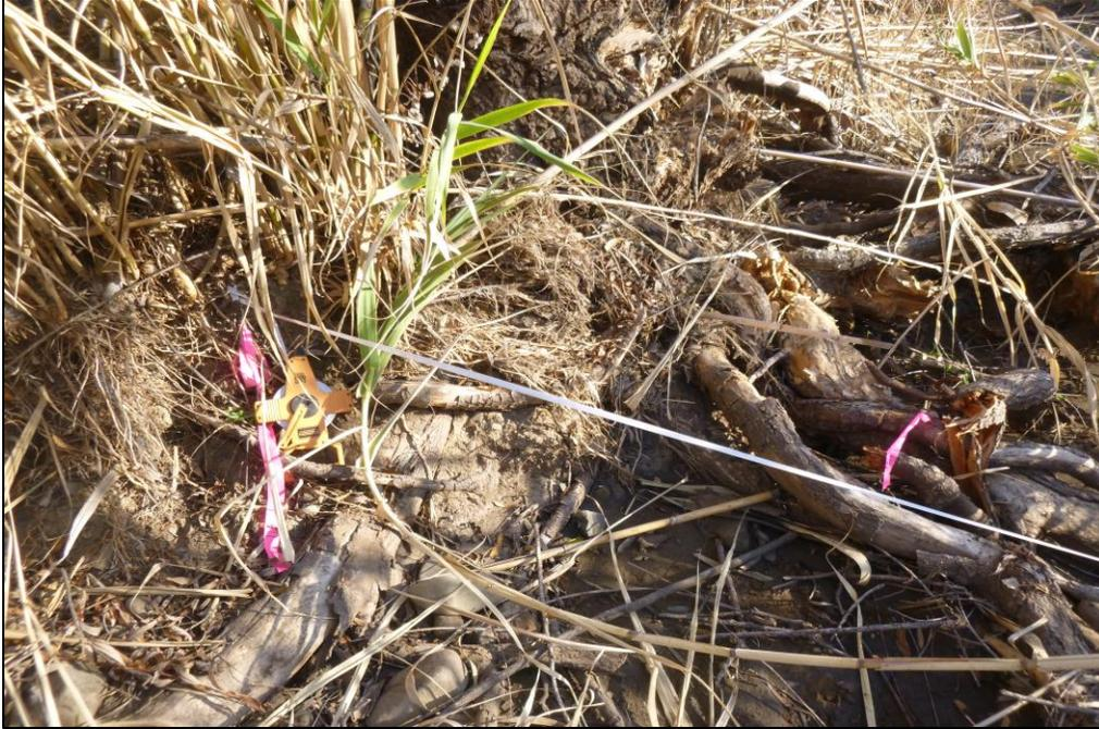
**Figure A-1.** Vertical benchmark driven into tree root near transect tail pin. The vertical benchmark and tail pin are marked with flagging tape.
