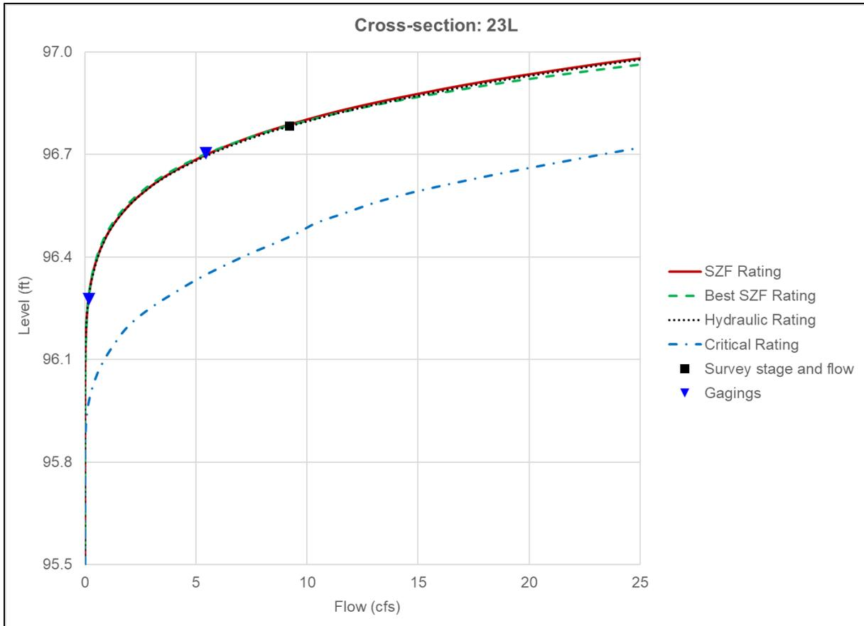
**Figure B-2.** Rating curve outputs for Reach 1, cross section 23L.
