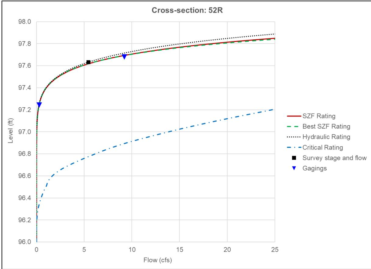
**Figure B-8.** Rating curve outputs for Reach 1, cross section 52R.
