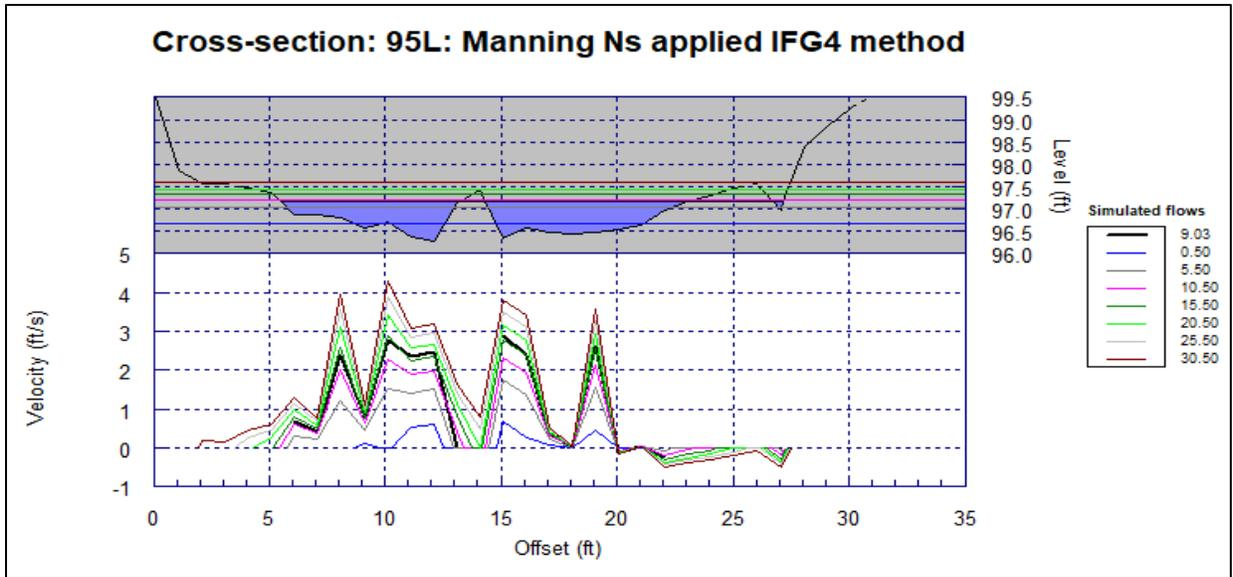
**Figure D-16.** Cross section 95L at simulated flows ranging from 0.5 cfs to 30.5 cfs.
