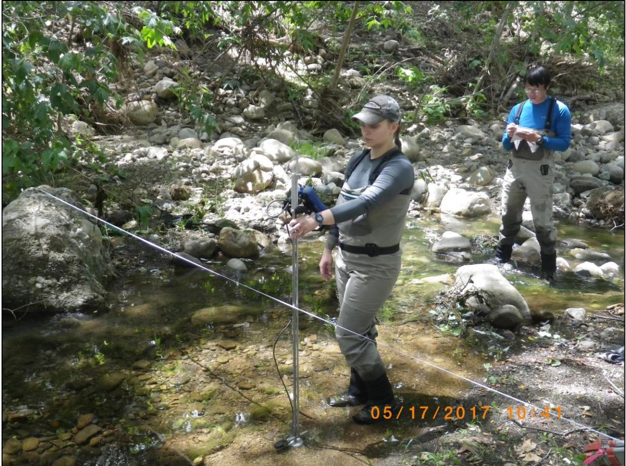
**Figure A-4.** Discharge measurement in San Antonio Creek Reach 2, flow pictured at approximately 0.4 cfs.
