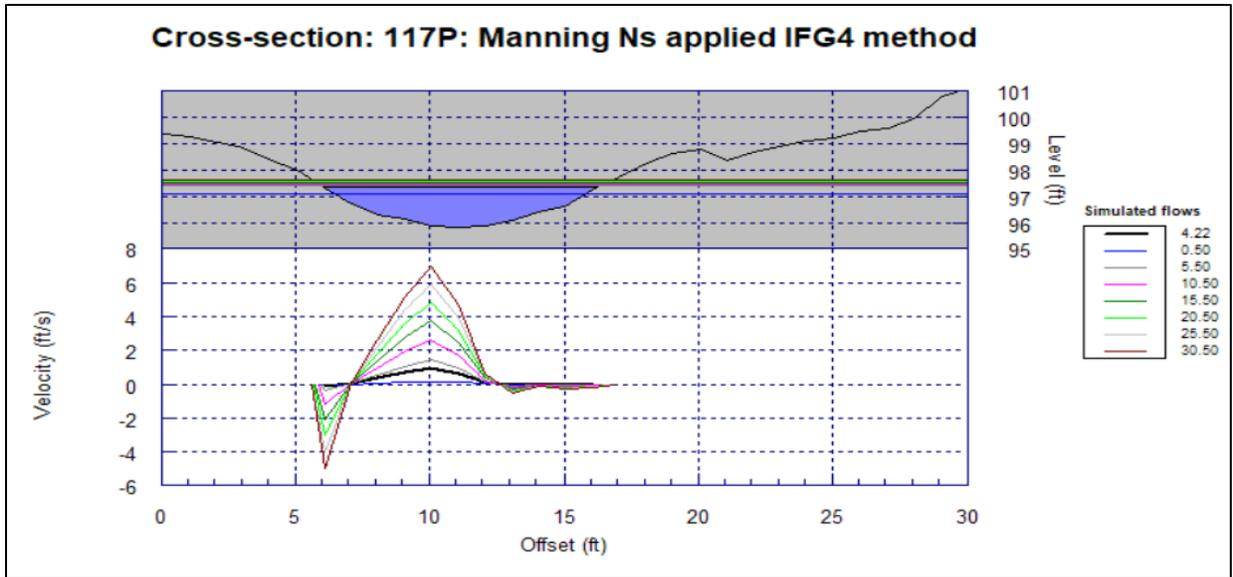
**Figure D-18.** Cross section 117P before VDF modification at simulated flows ranging from 0.5 cfs to 30.5 cfs.
