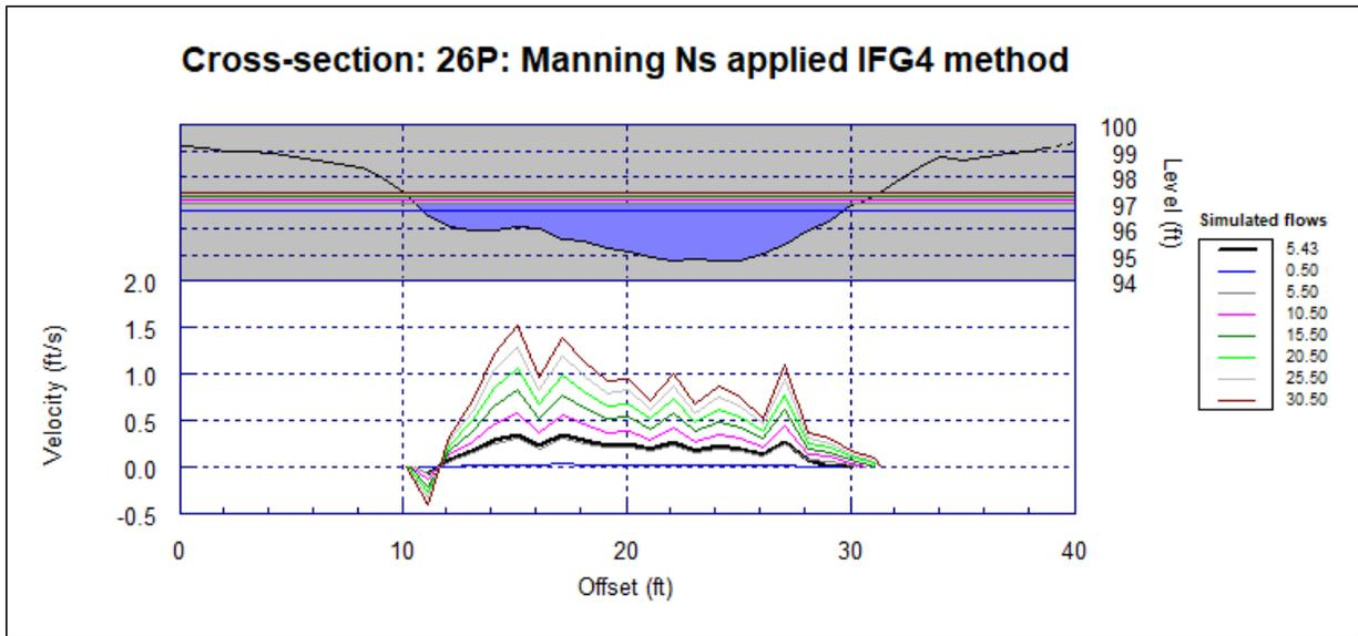
**Figure D-3.** Cross section 26P at simulated flows ranging from 0.5 cfs to 30.5 cfs.
