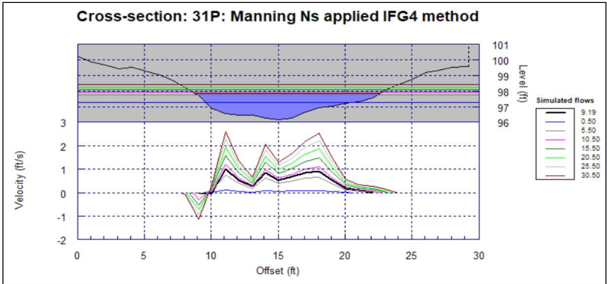
**Figure D-6.** Cross section 31P before VDF modification at simulated flows ranging from 0.5 cfs to 30.5 cfs.
