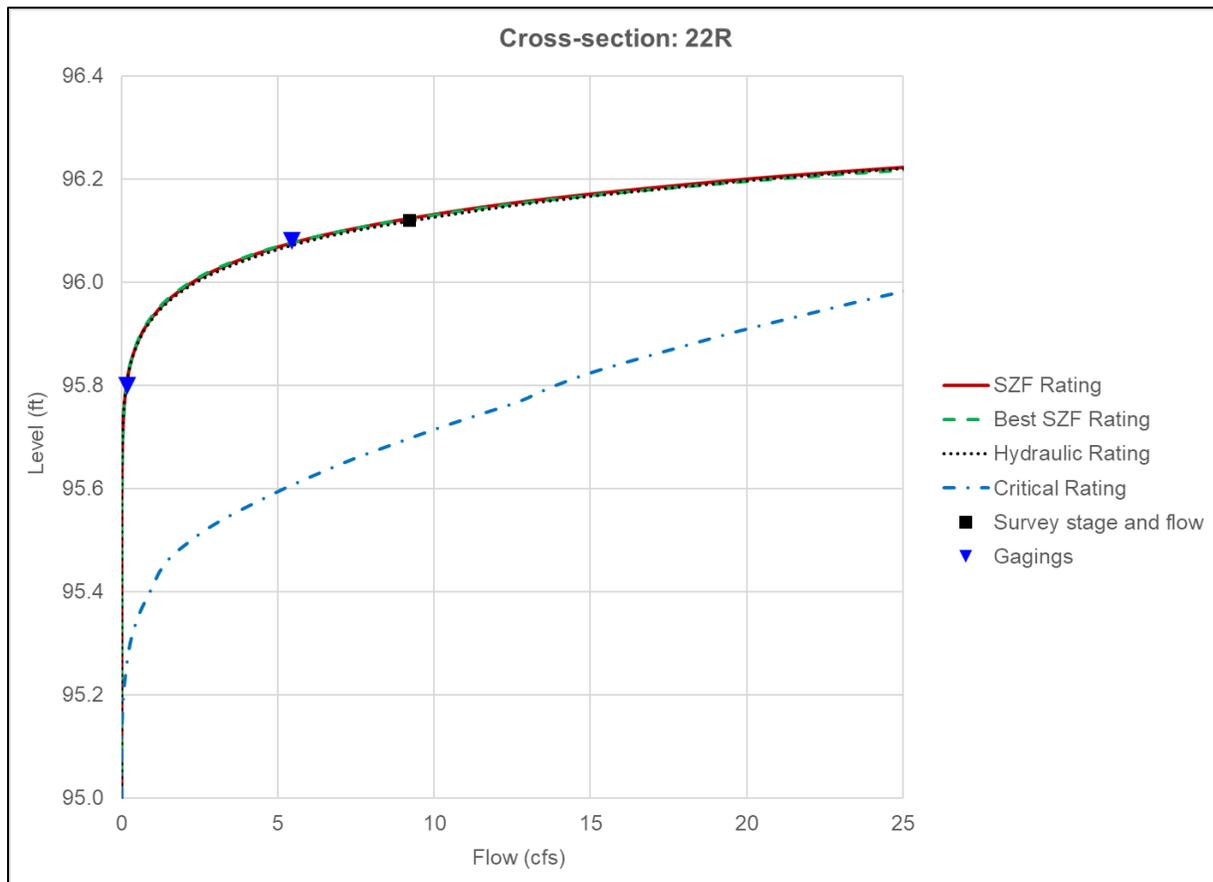
Figure B-1. Rating curve outputs for Reach 1, cross section 22R.
