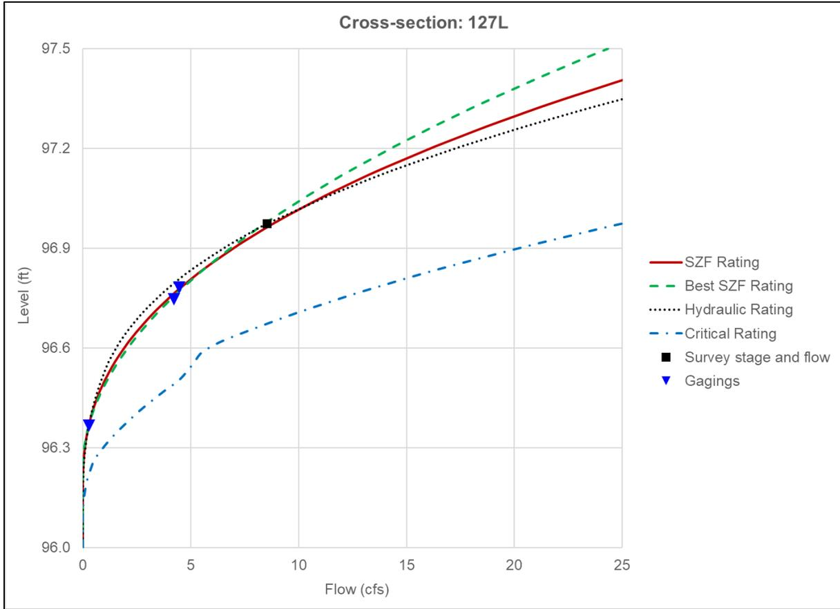
**Figure B-15.** Rating curve outputs for Reach 2, cross section 127L.
