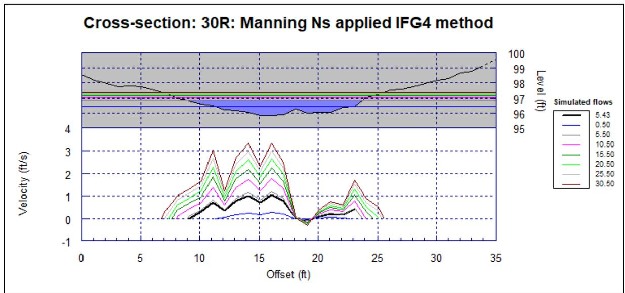
**Figure D-5.** Cross section 30R at simulated flows ranging from 0.5 cfs to 30.5 cfs.
