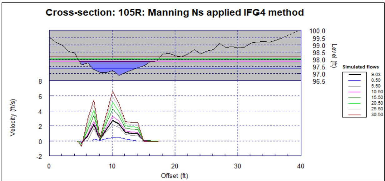
**Figure D-17.** Cross section 105R at simulated flows ranging from 0.5 cfs to 30.5 cfs.
