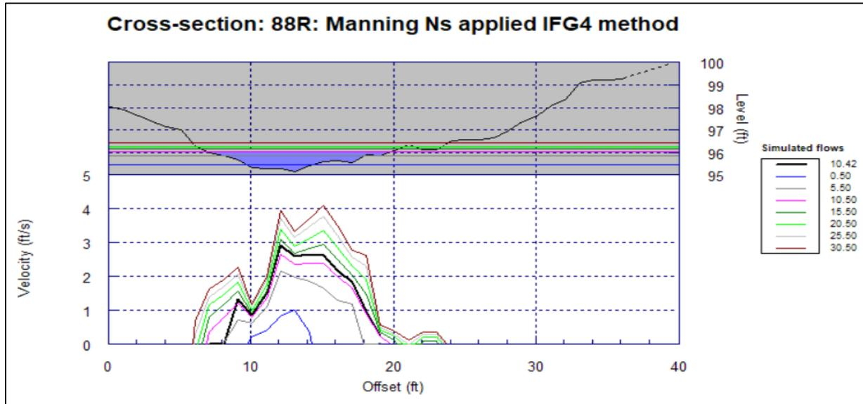
**Figure D-12.** Cross section 88R before VDF modification at simulated flows ranging from 0.5 cfs to 30.5 cfs.
