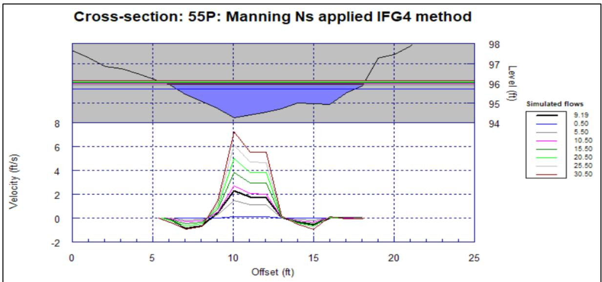
**Figure D-11.** Cross section 55P after VDF modification at simulated flows ranging from 0.5 cfs to 30.5 cfs.
