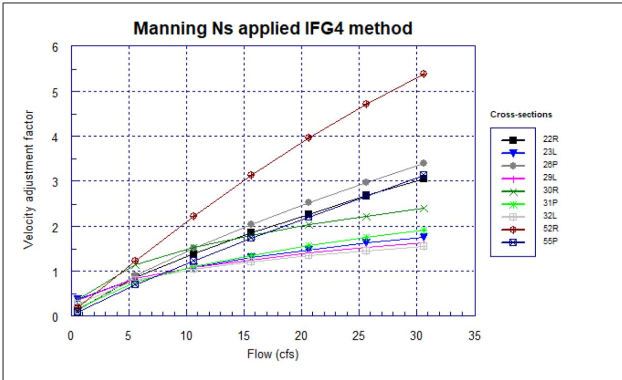
Figure A-9. Velocity simulation VAFs by discharge in Reach 1.
