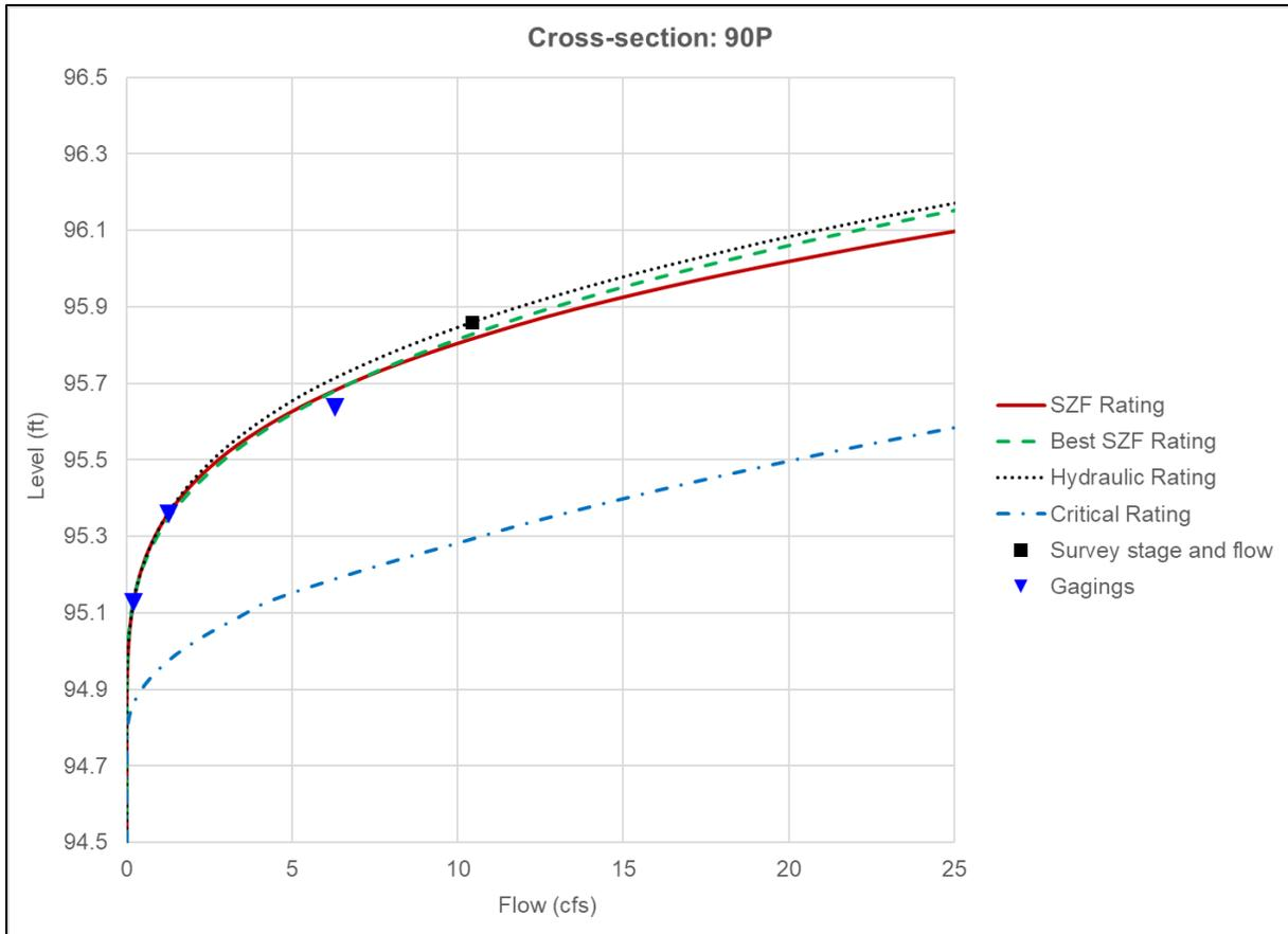
**Figure B-11.** Rating curve outputs for Reach 2, cross section 90P.
