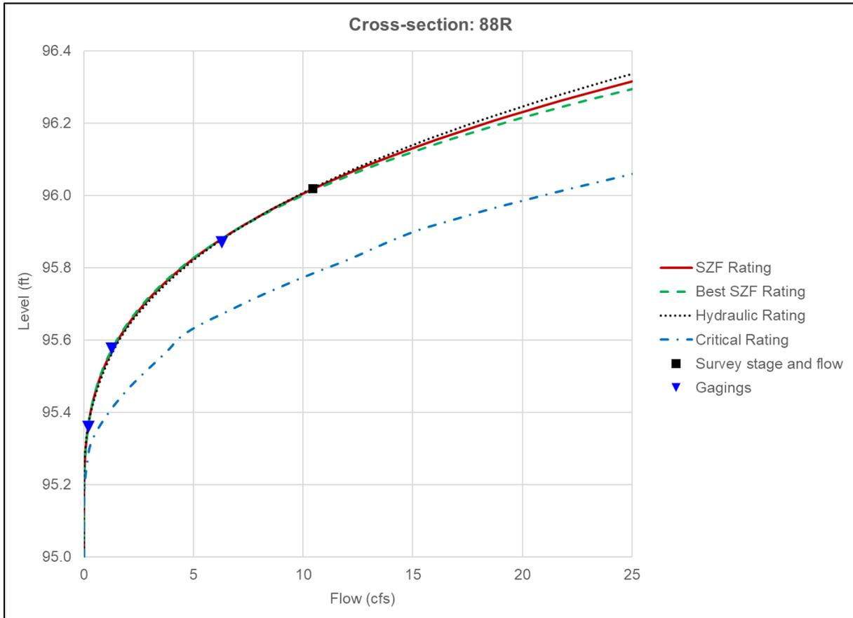
**Figure B-10.** Rating curve outputs for Reach 2, cross section 88R.
