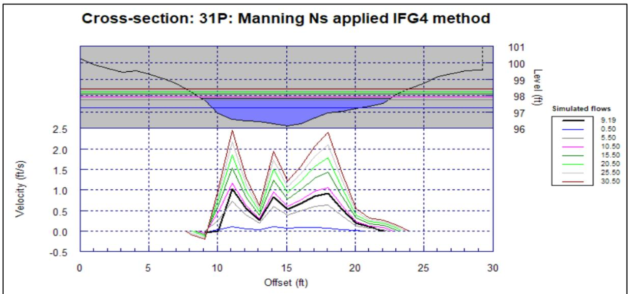
**Figure D-7.** Cross section 31P after VDF modification at simulated flows ranging from 0.5 cfs to 30.5 cfs.
