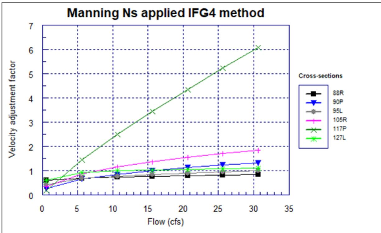
Figure A-10. Velocity simulation VAFs by discharge in Reach 2.
