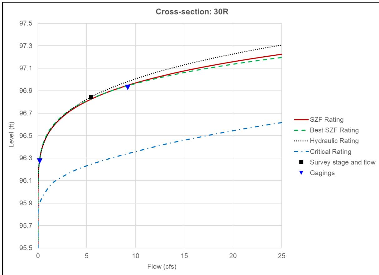
**Figure A-5.** Example SEFA rating curve output. Rating curves for additional transects are in Appendix B.
