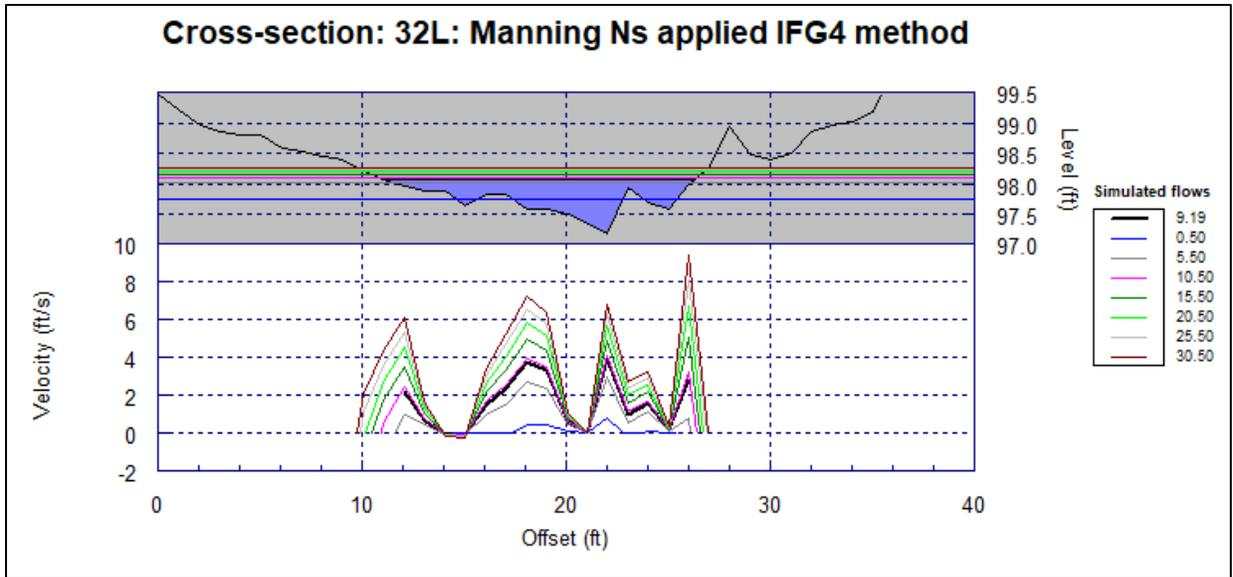
**Figure D-8.** Cross section 32L at simulated flows ranging from 0.5 cfs to 30.5 cfs.
