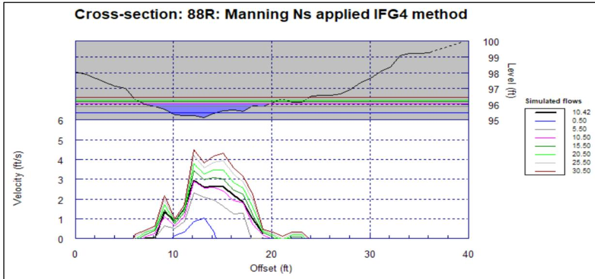
**Figure D-13.** Cross section 88R after VDF modification at simulated flows ranging from 0.5 cfs to 30.5 cfs.
