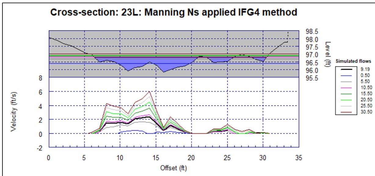
**Figure D-2.** Cross section 23L at simulated flows ranging from 0.5 cfs to 30.5 cfs.
