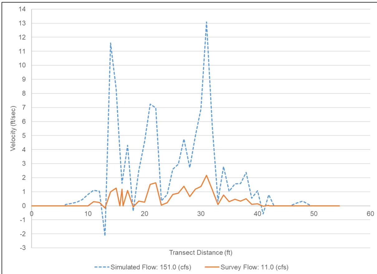
**Figure A-7.** Example simulation of small negative velocities in SEFA. Velocities increase in negative magnitude at higher simulated flow levels.
