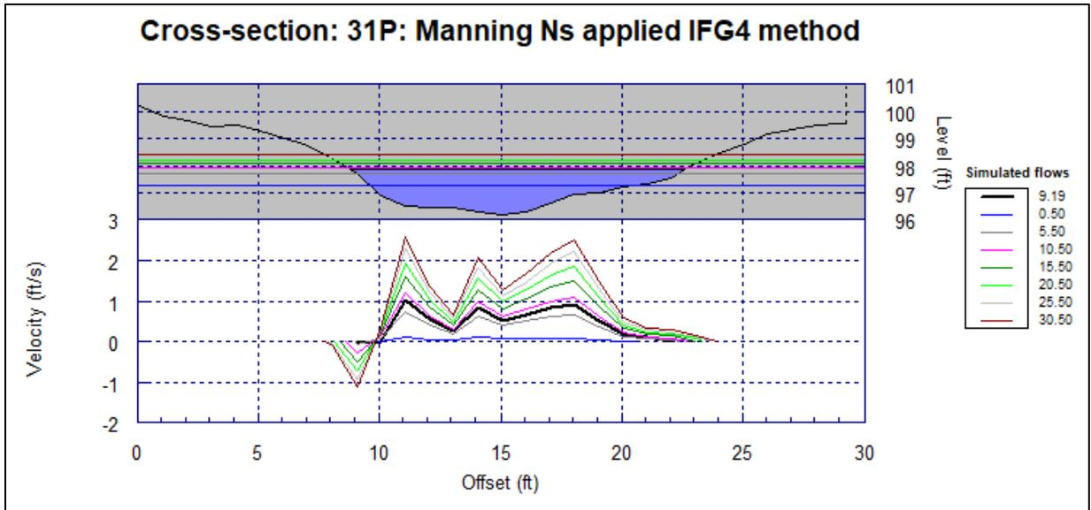
**Figure A-8.** Example transect showing the pattern of the simulated velocities. On this transect, the simulated velocities do not follow the trend of the field-measured velocity profile, bold black line, at offset 9 and 10.
