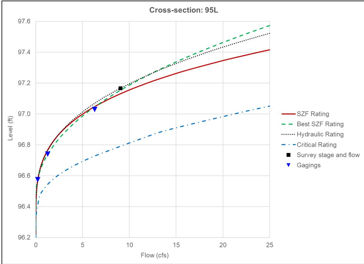
**Figure B-12.** Rating curve outputs for Reach 2, cross section 95L.
