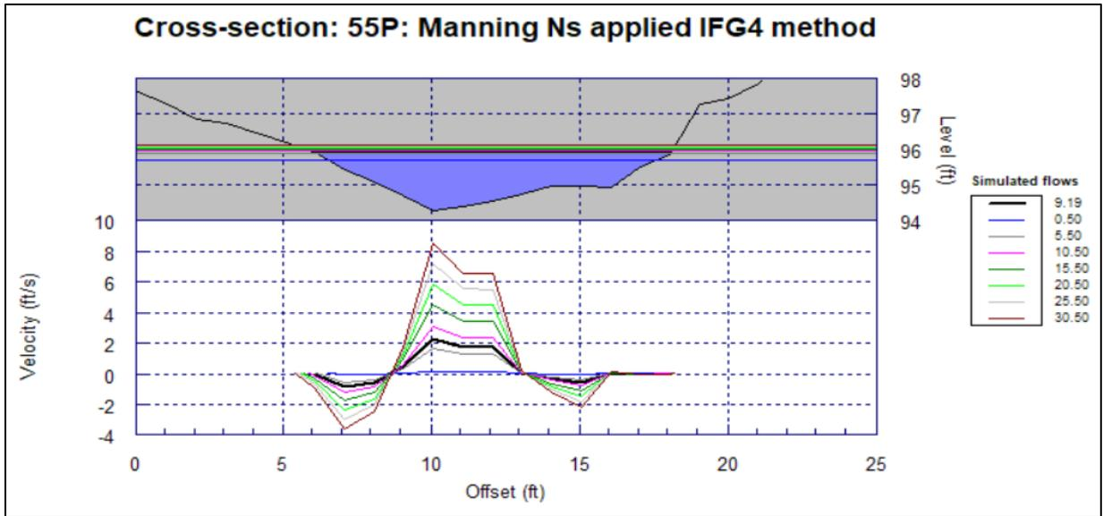
**Figure D-10.** Cross section 55P before VDF modification at simulated flows ranging from 0.5 cfs to 30.5 cfs.
