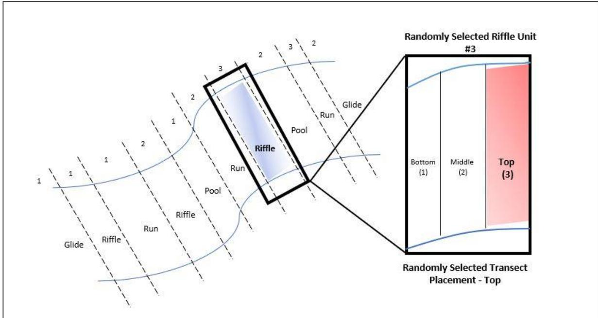
**Figure 14.** Schematic of mesohabitat unit site selection and transect placement.
