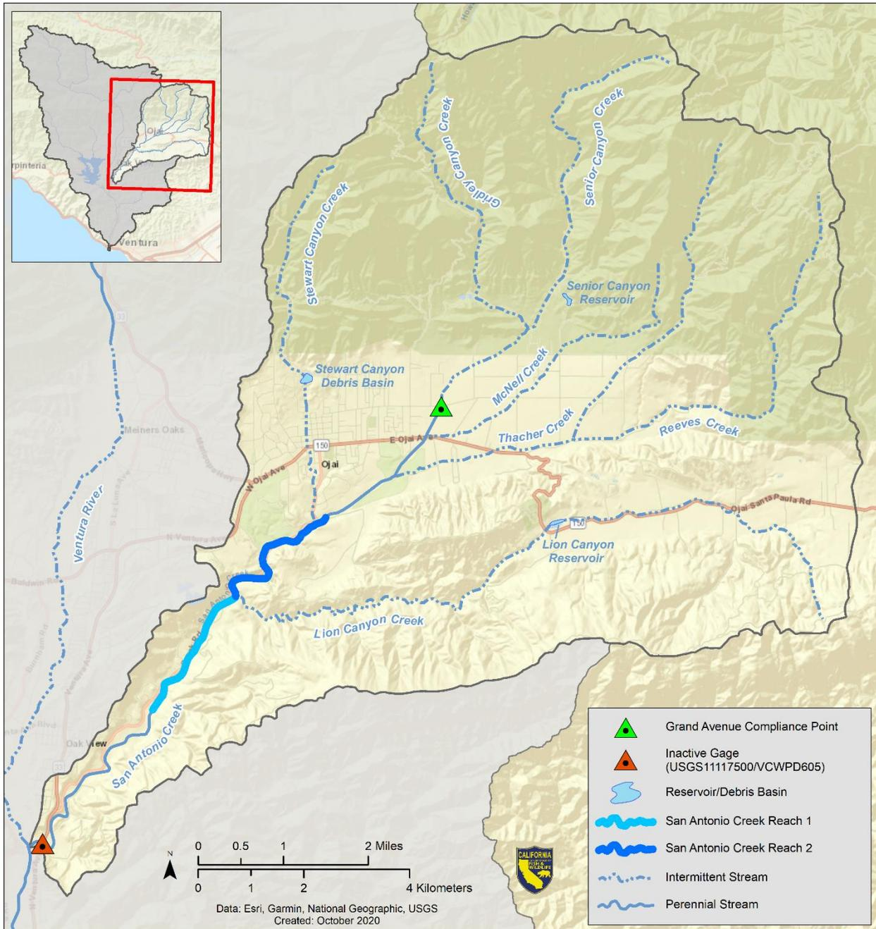
**Figure 3.** Map of San Antonio Creek watershed. Note: intermittent and perennial streams shown here were classified by the United States Geological Survey (USEPA and USGS 2012). An active gage (VCWPD 605A), not used in this report, is located just upstream of the mapped inactive gage.
