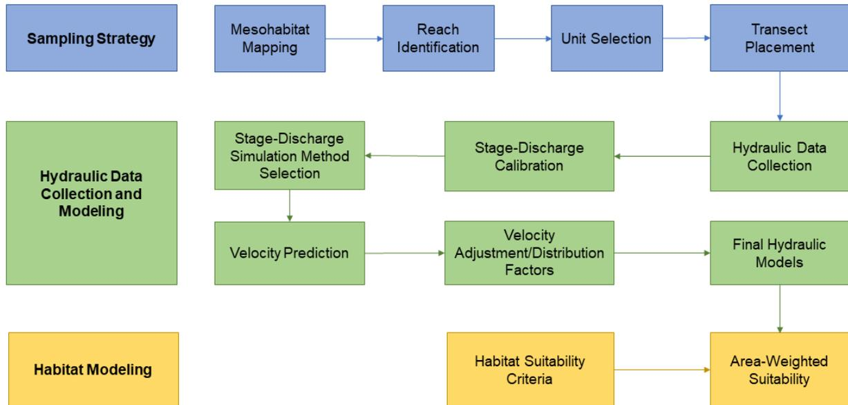
**Figure 12.** General schematic of 1D model development for physical habitat simulation.
