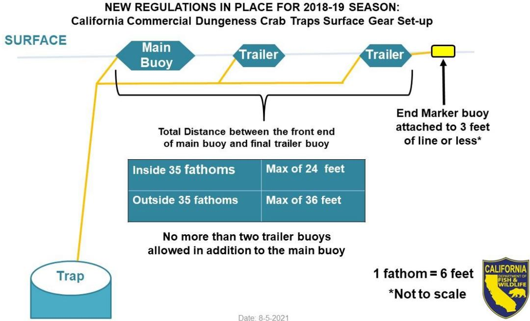
Figure 2-4. Schematic showing surface gear restrictions in place as of October 2018. Credit: CDFW.
