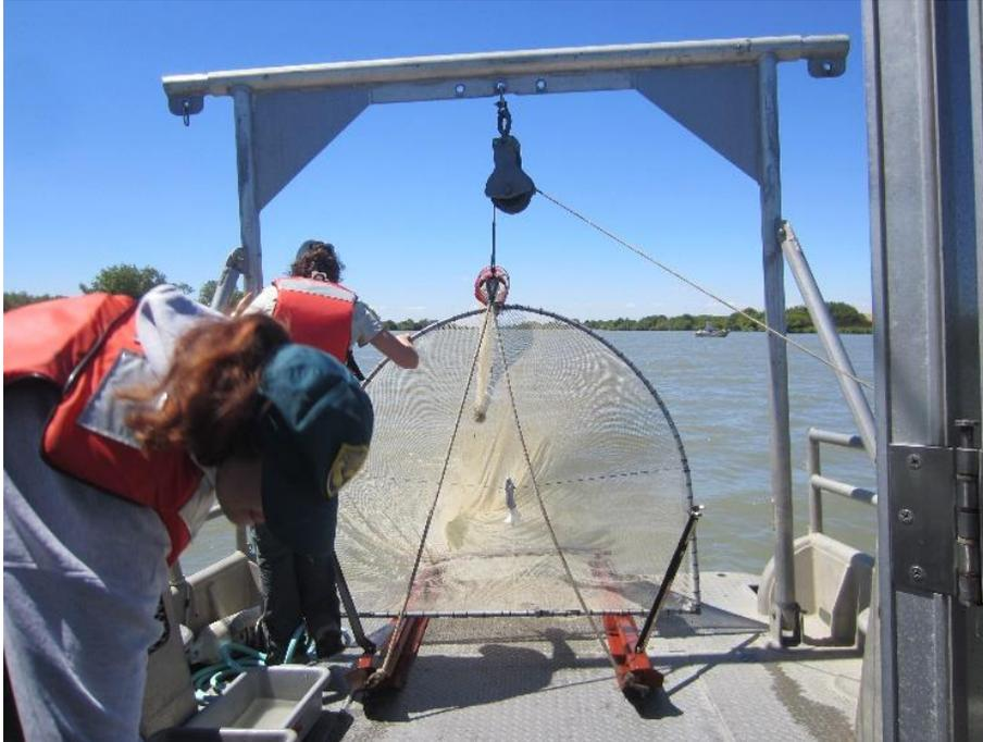
Figure 3. The tow net in the field ready for deployment. Note flowmeter in center of net mouth with CB net attached on top of the D-ring frame.
