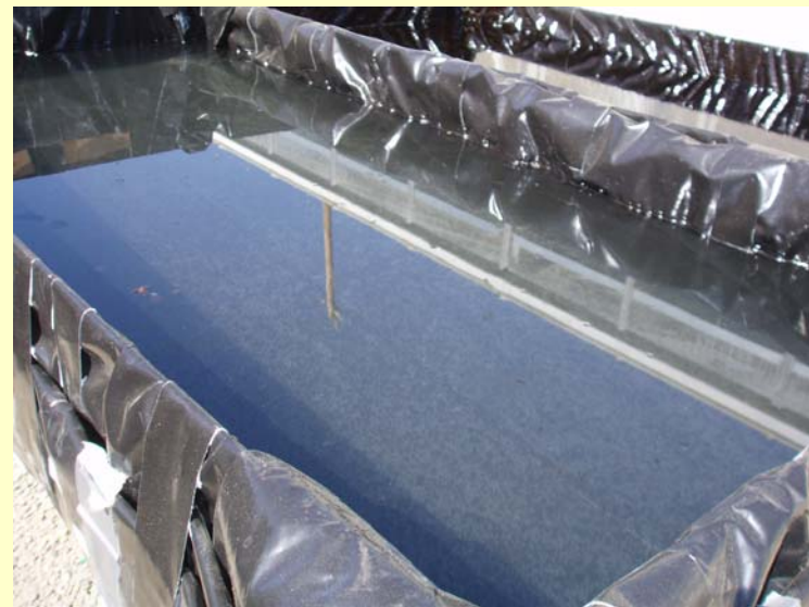
After diesel oil application: Sorbent on left and No Sorbent on right
