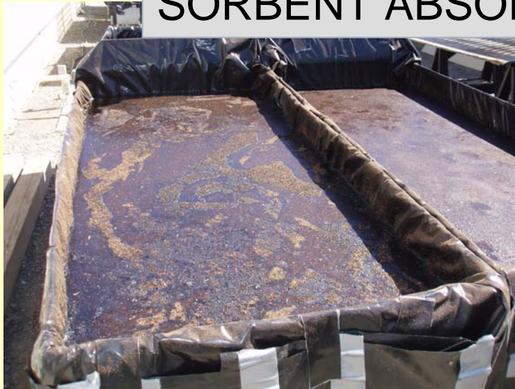
After PBC application: Sorbent on left and No Sorbent on right
