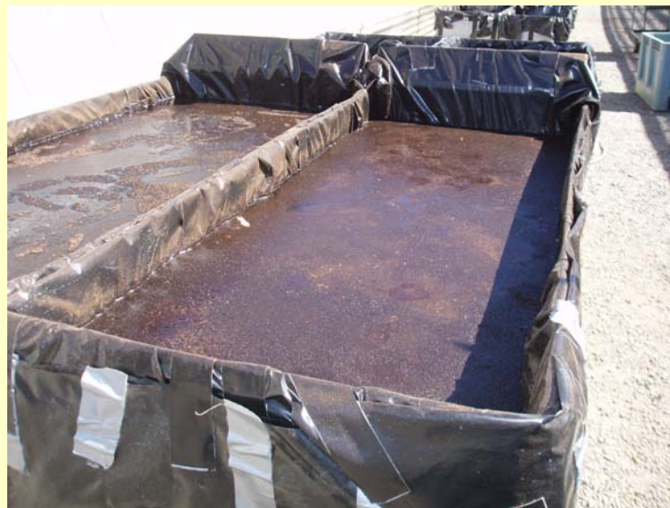
After diesel oil application: Sorbent on left and No Sorbent on right
