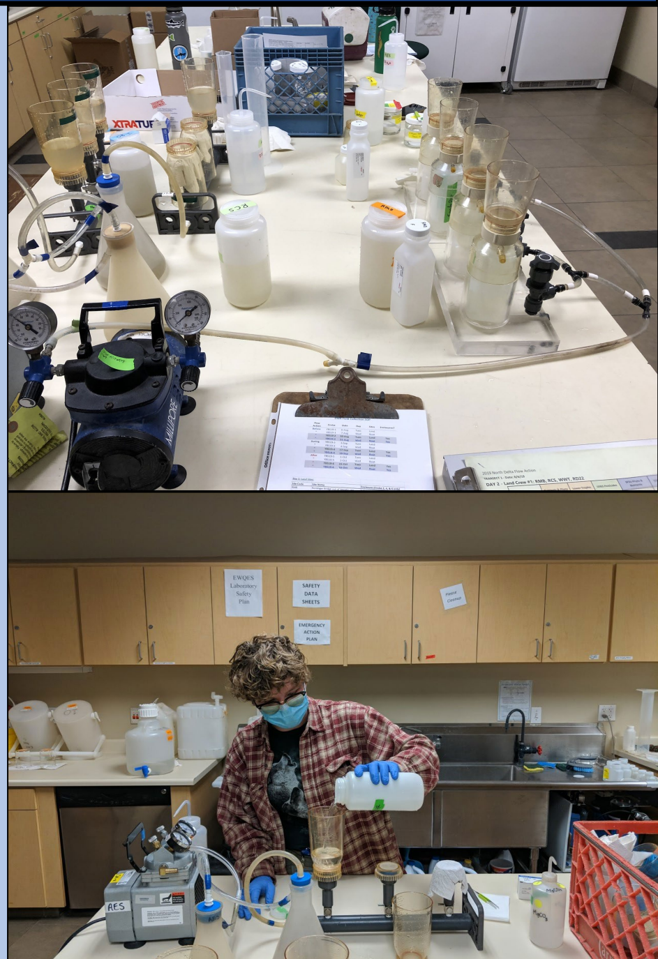
Top: Set up of our filtration stations in the lab Bottom: Using filtering equipment to filter for chlorophyll-a
