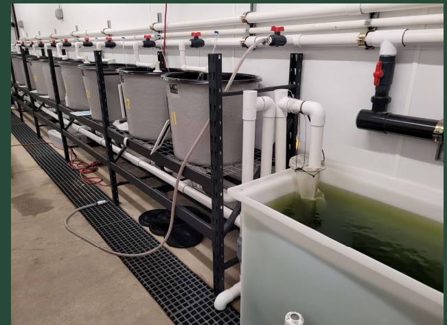
New late-larval (41–80 dph) rearing system.
