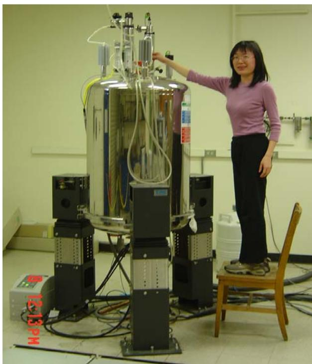
Figure 25. Avance DRX-500 NMR spectrometer.
