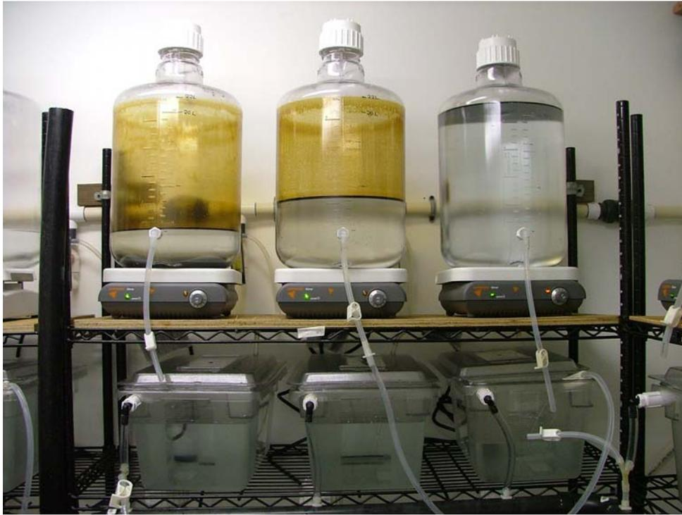
Figure 24 . 20-L polycarbonate carboys used for WAF and CEWAF preparation (above) and 18-L polycarbonate aquaria used for smolt exposures (below).
