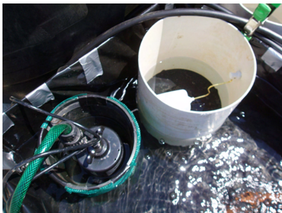
Fig. 3. Submersible pump in well, and float-shutoff for water height control before adding Perlite.
