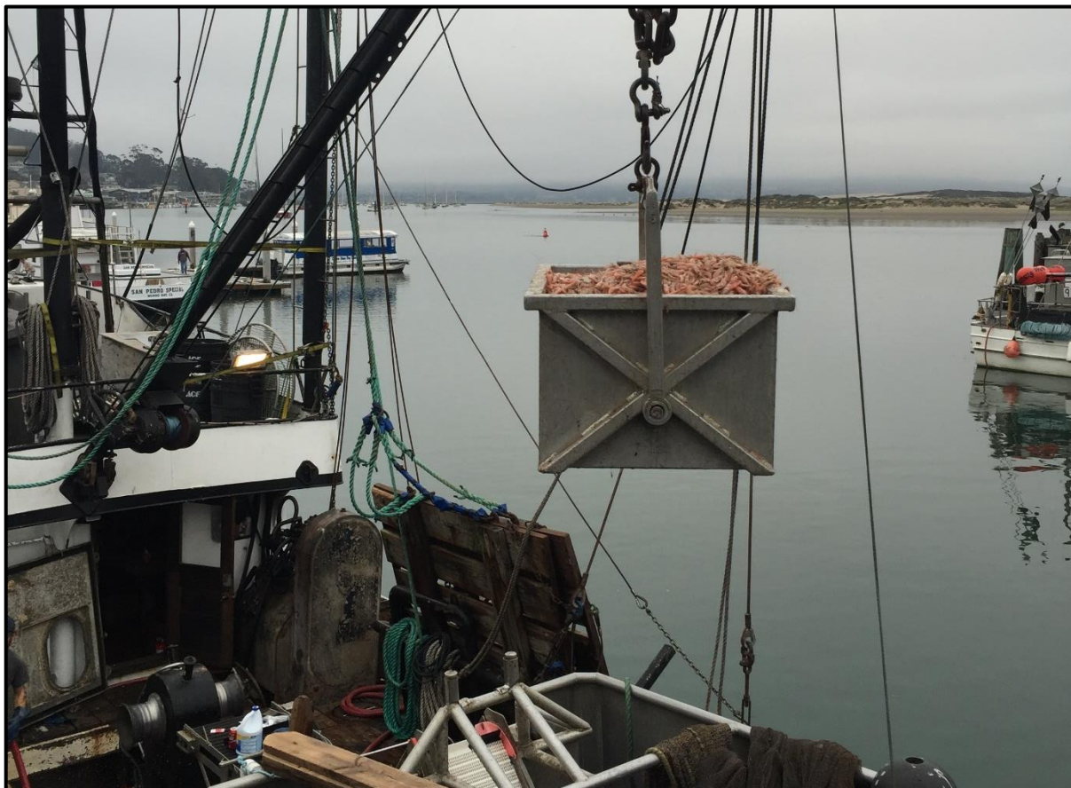
Figure 7. Photo of a bucket hoist transferring shrimp from a vessel (Credit: J. Grebel).
