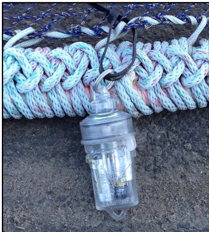
Figure 3. Picture of an FLD attached to the footrope of a trawl net (Credit: J. Grebel).
