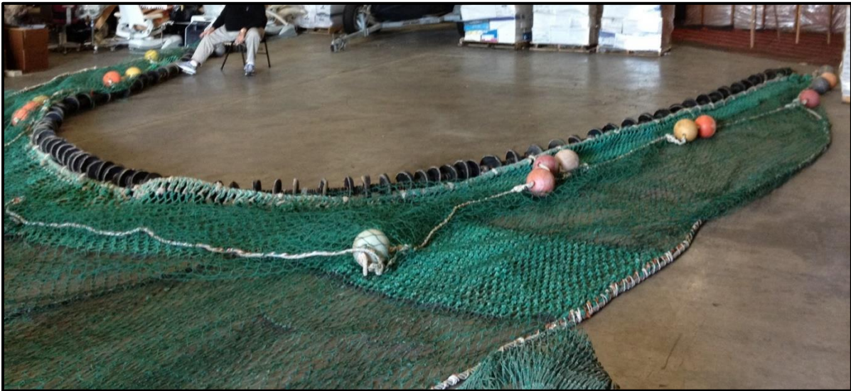
Figure 5. A pink shrimp trawl net with its width arranged in a “U” shape. An individual can be seen seated near the top left corner of the photo for size comparison (Credit: J. Grebel).
