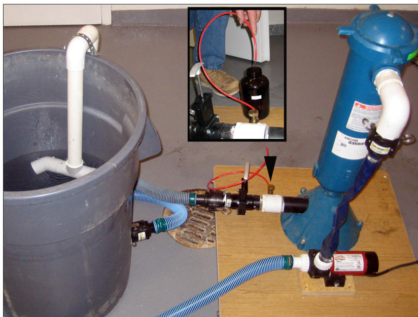
Fig 2. In trials 2 and 3, water samples were collected (see insert) using a small brass valve (black arrow).
