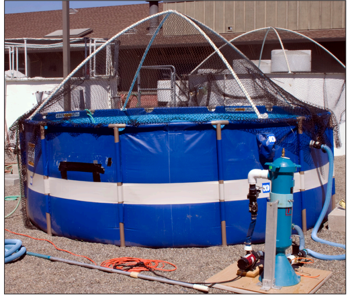
Fig 3. X100 filter connected to temporary rehabilitation pool.
