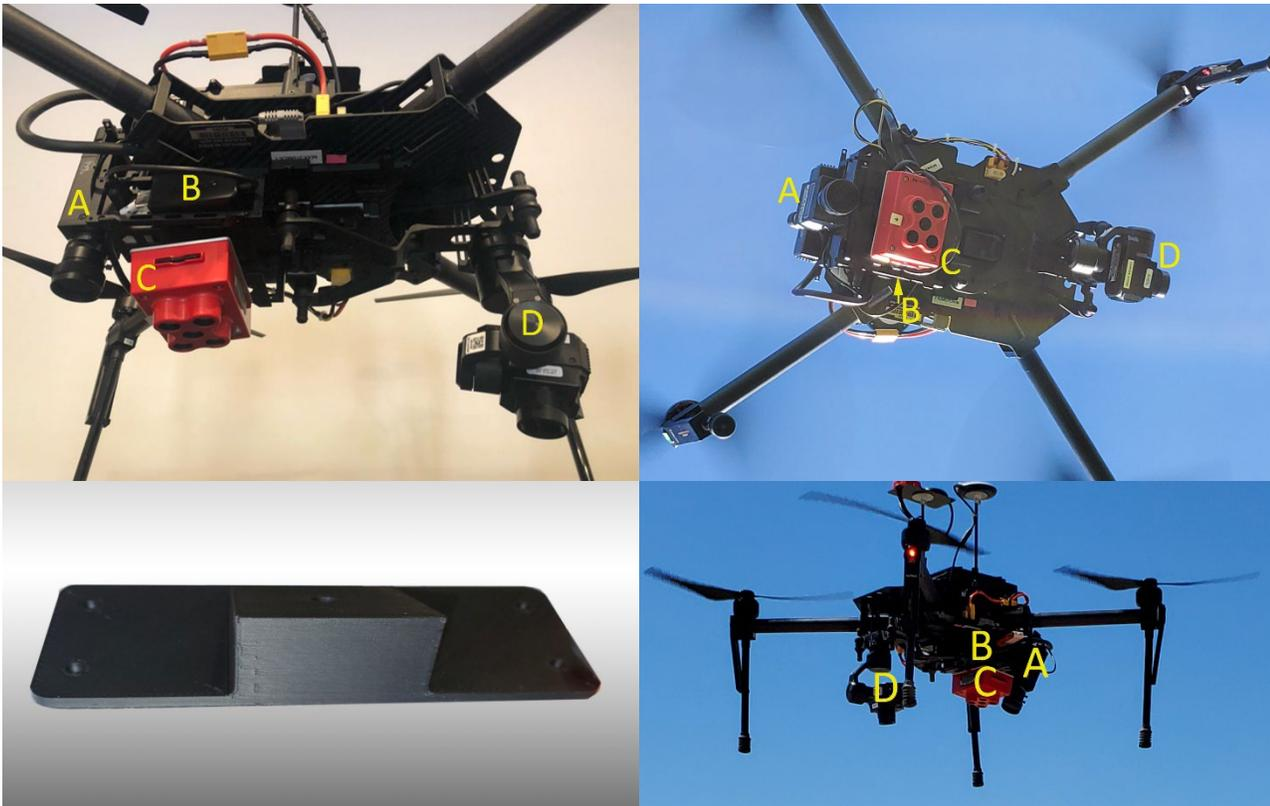
Figure 1. M100 with camera systems and SBC installed (A=JAI CM-140GE-UV, B=RPI SBC, C=MicaSense RedEdge MS, D= Zenmuse XT TIR). Bottom left image shows custom mount for UV camera (B). Bottom right image shows final camera alignment and SBC placement.
