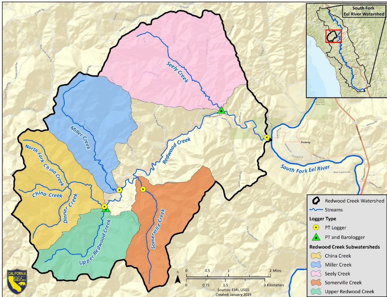
**Figure 3.** Barologger and pressure transducer (PT) locations within the study area.
