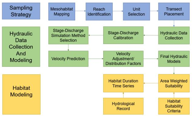
Figure 7. General schematic of 1D model development for physical habitat simulation.
