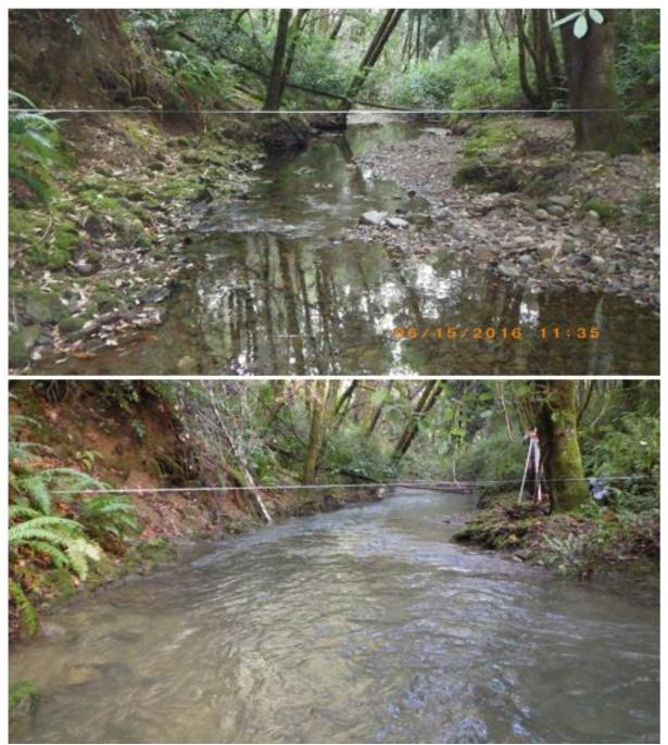
**Figure 24.** Downstream view of transect URT25 (Upper Redwood Creek) at 0.5 cfs (top) and 26.6 cfs (bottom).
