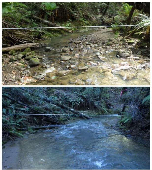
**Figure 30.** Downstream view of transect NFCT25 (North Fork China Creek) at 0.4 cfs (top) and 7.3 cfs (bottom).
