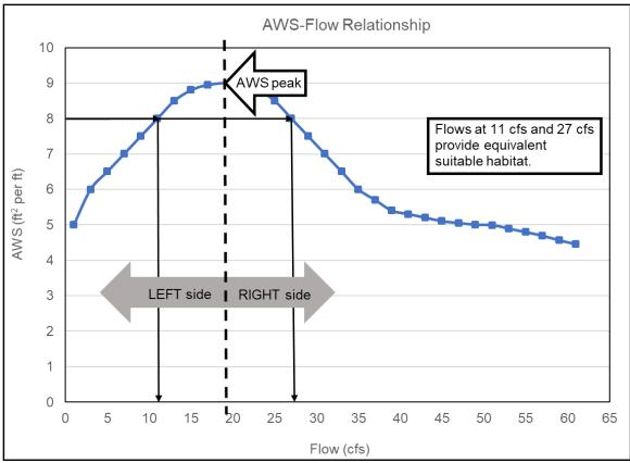
**Figure 11.** An example of an AWS-flow relationship; the same amount of suitable habitat can be provided by flows both above and below the AWS peak flow.
