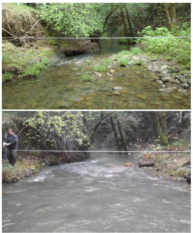
**Figure 27.** Downstream view of transect MCT17 (Miller Creek) at 3.6 cfs (top) and 32 cfs (bottom).
