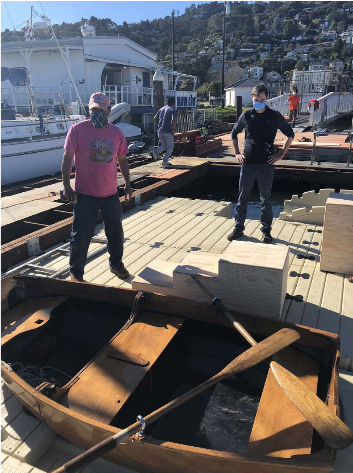
Image 4: Photo of a small el-toro sailboard demonstrating the transfer bench steps. The gap between the plastic and wooden docks behind it is where the small aluminum ramp was placed (Photo credit: Sausalito Community Boating Center).
