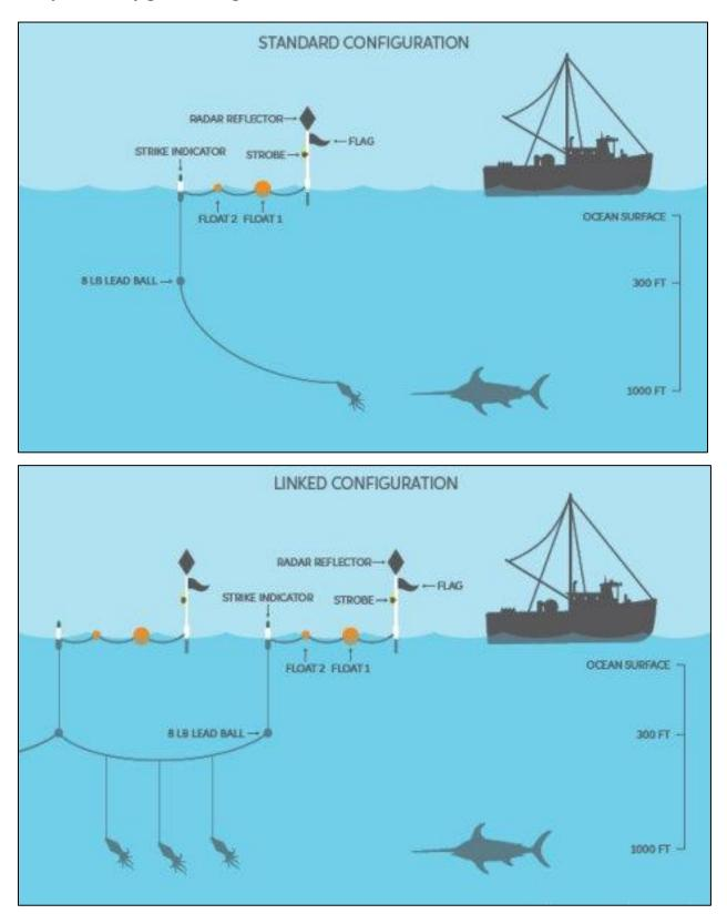
Night-set buoy gear configuration (*light color has been changed to blue on actual gear at request of Enforcement*):
