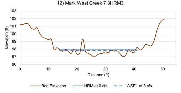
Figure B-13. Mark West Creek 3HRM3 transect cross section with bed elevation, WPM WSEL, and HRM WSEL.
