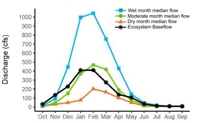
Figure 5. Ecosystem baseflows and median natural flows (Mark West Creek 1).
