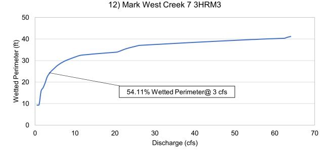
Figure B-14. Mark West Creek 3HRM3 transect wetted perimeter-discharge curve.
