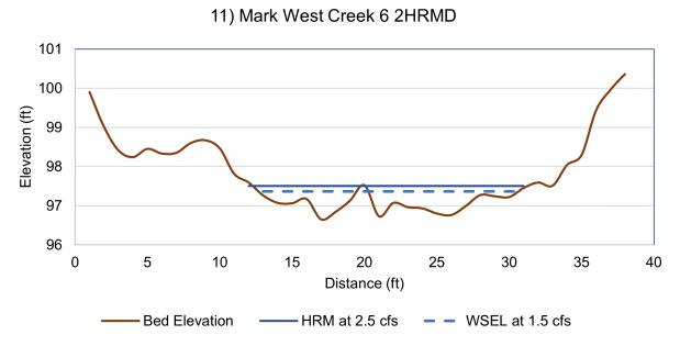
Figure B-5. Mark West Creek 2HRMD transect cross section with bed elevation, WPM WSEL, and HRM WSEL.
