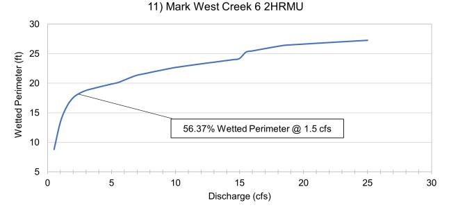
Figure B-10. Mark West Creek 2HRMU transect wetted perimeter-discharge curve.
