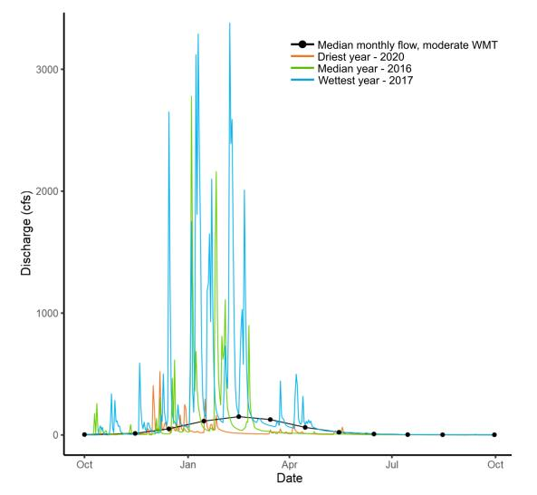
Figure 4. Variation in mean daily Santa Rosa Creek flows at USGS gage 11466320, located in the Mark West Creek watershed, in extreme and median conditions (i.e., the driest, median, and wettest year) between water years 2000 and 2021 (USGS 2022). Median monthly flow for a moderate water month type (WMT) is also included.
