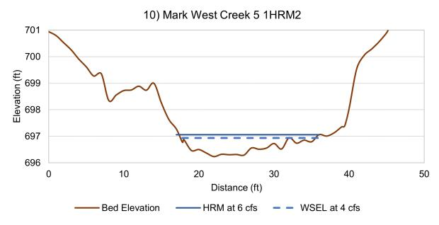
Figure B-3. Mark West Creek 1HRM2 transect cross section with bed elevation, WPM WSEL, and HRM WSEL.
