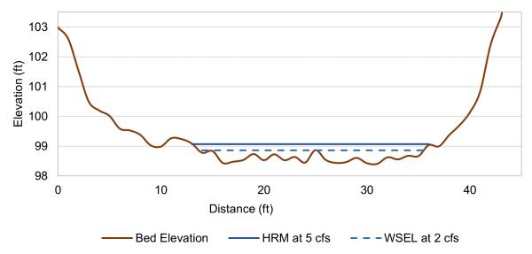
Figure B-1. Mark West Creek 1HRM1 transect cross section with bed elevation, WPM WSEL, and HRM WSEL.
