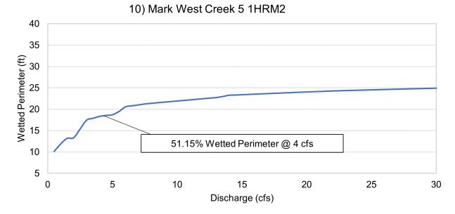
Figure B-4. Mark West Creek 1HRM2 transect wetted perimeter-discharge curve.
