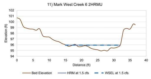
Figure B-9. Mark West Creek 2HRMU transect cross section with bed elevation, WPM WSEL, and HRM WSEL.
