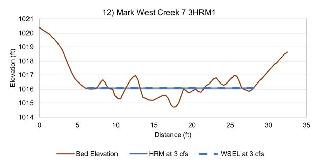
Figure B-11. Mark West Creek 3HRM1 transect cross section with bed elevation, WPM WSEL, and HRM WSEL.
