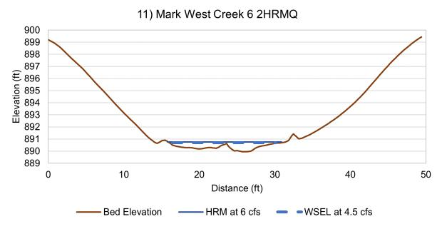
Figure B-7. Mark West Creek 2HRMQ transect cross section with bed elevation, WPM WSEL, and HRM WSEL.
